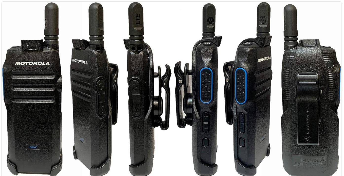
Figure 2: Various angles of the Motorola TLK100 radio, including views of the side PTT button, top controls, and the attached belt clip. This illustrates the ergonomic design and accessory options.
