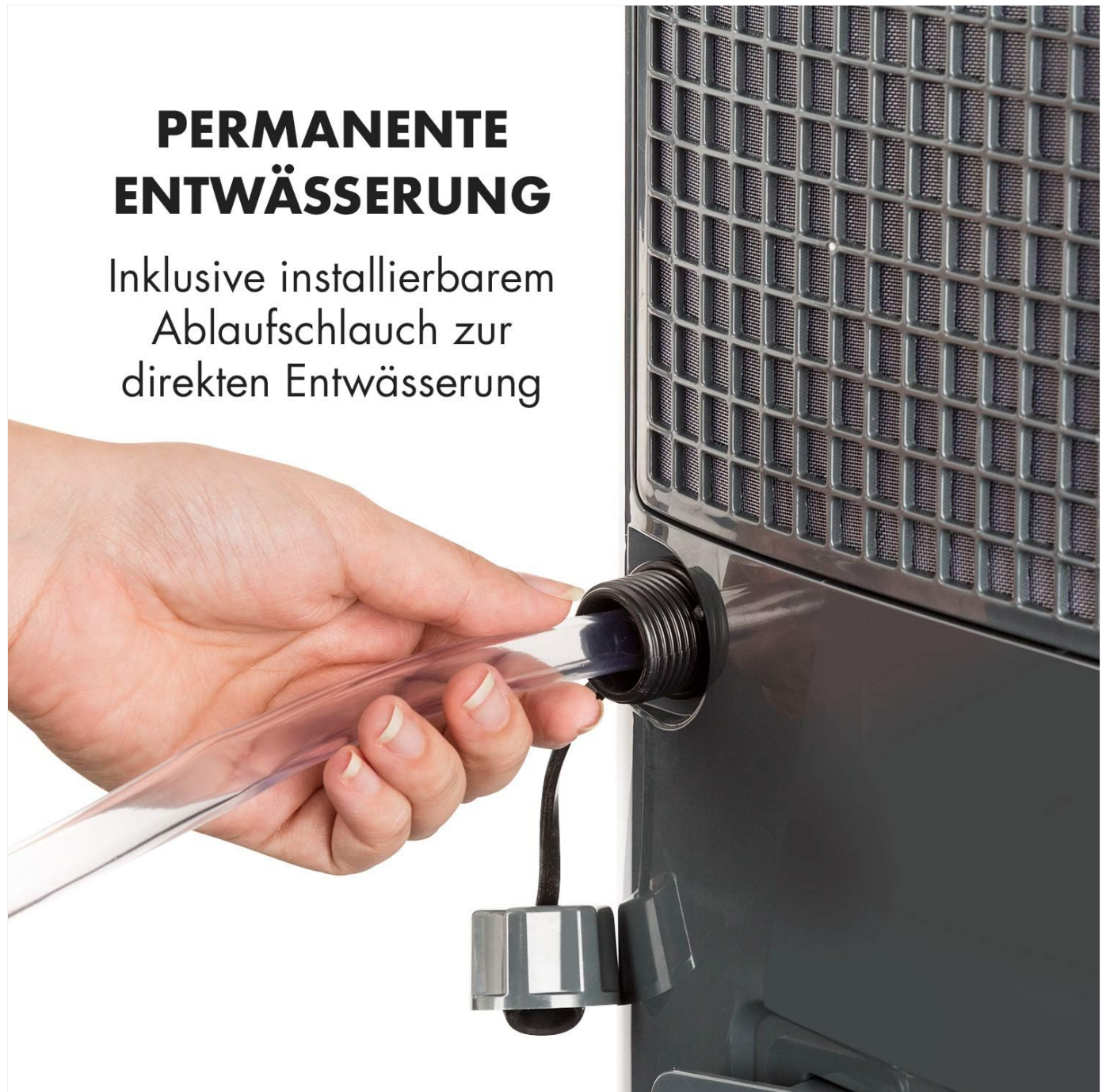
Image 5.2: The continuous drainage feature allows for extended operation by directing collected water through a hose to a drain, eliminating the need to manually empty the tank.
