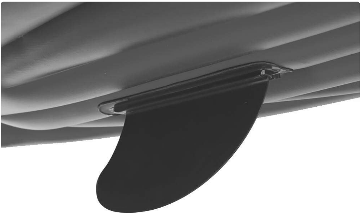
Figure 4.4: Removable skeg for directional stability.
