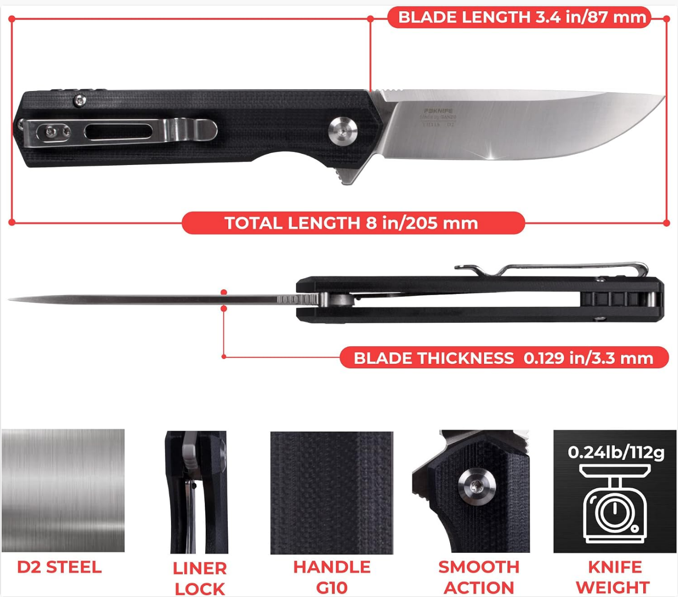
Image 8.1: Detailed dimensions and material specifications of the knife.
