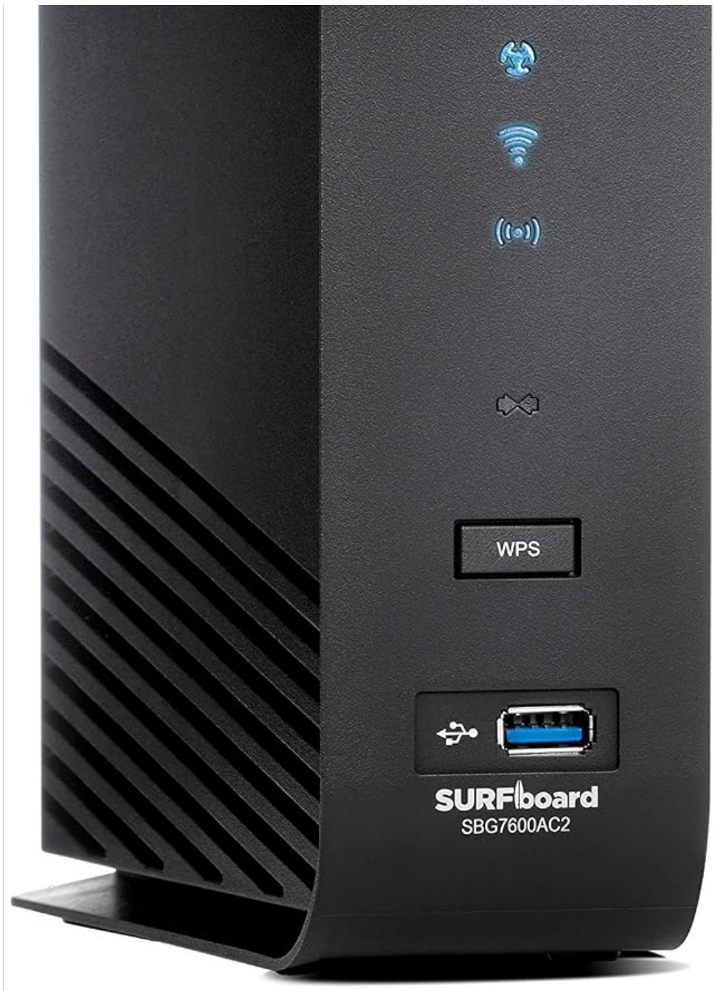
Image 3.1: Front view of the ARRIS SBG7600AC2, displaying the vertical row of indicator lights and the WPS button.
