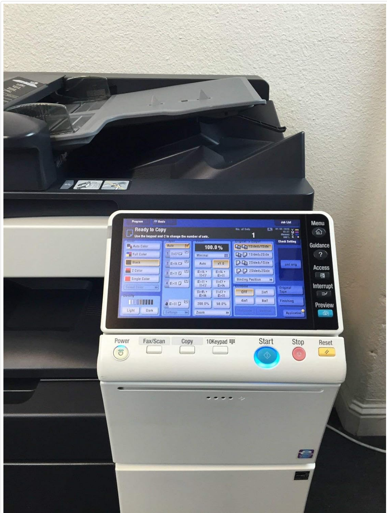
Figure 3.2: Close-up view of the Bizhub C364 control panel, featuring a large color touchscreen display, physical buttons for Power, Fax/Scan, Copy, 10-Keypad, Start, Stop, and Reset, and status indicators.
