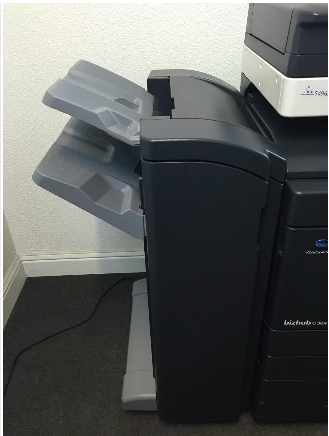
Figure 3.5: Side view of the Bizhub C364 showing the output tray, where printed or copied documents are collected.
