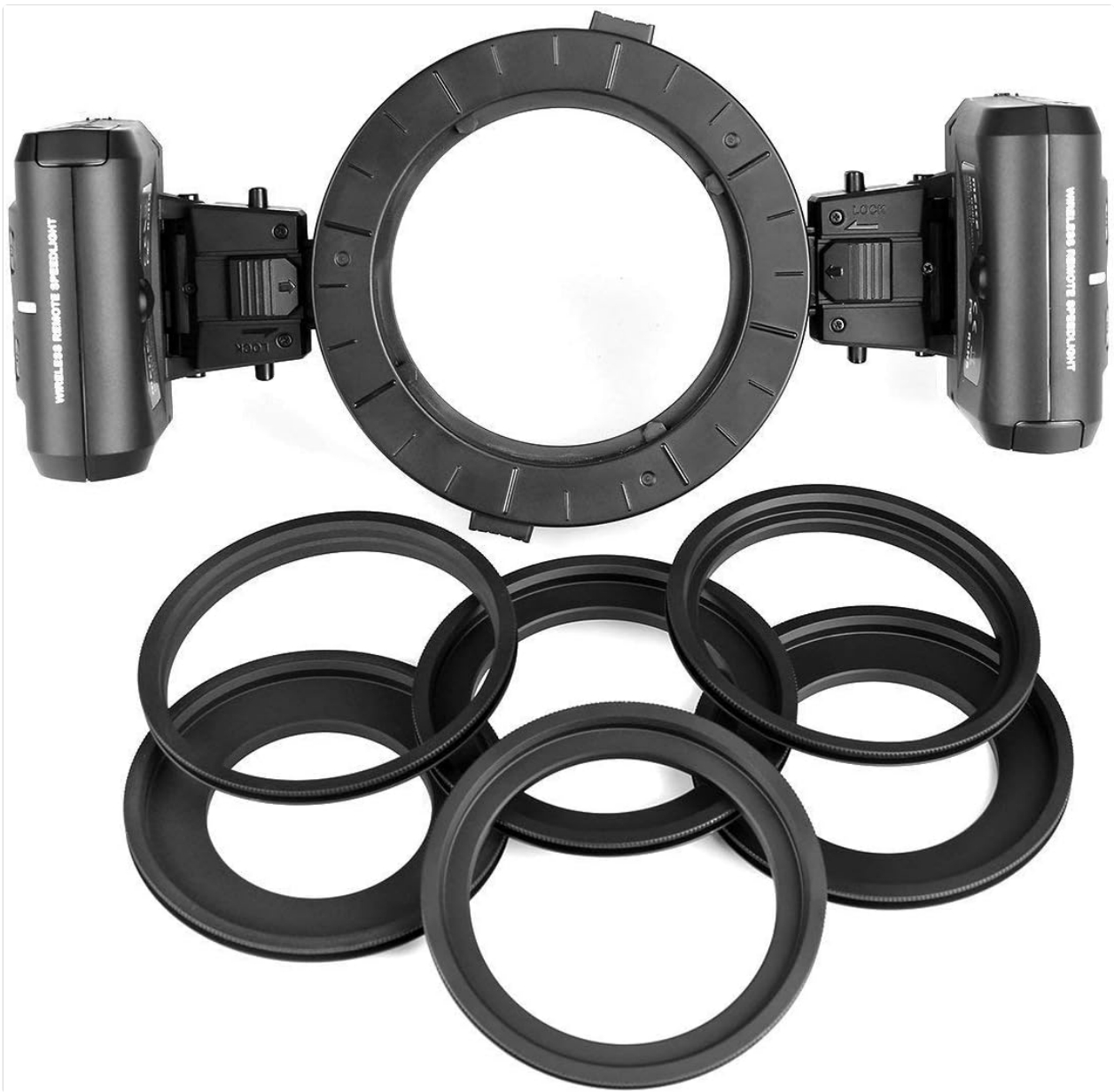
Figure 4.3: The MK-R200 flashes attached to the annular lamp holder, along with various lens adapter rings.
