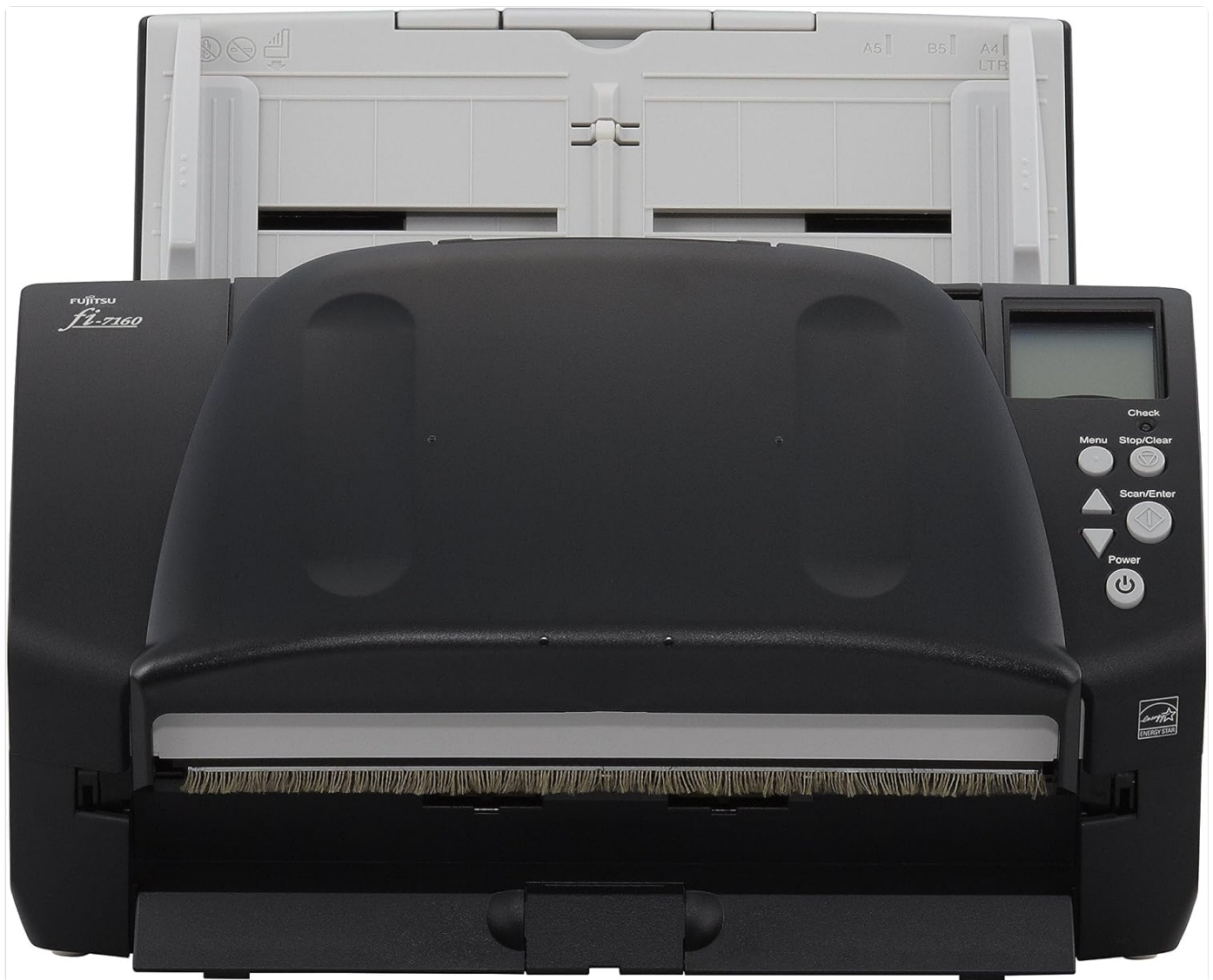
Figure 1: Front view of the Fujitsu Fi-7160 scanner, showing the paper input tray and control panel.
