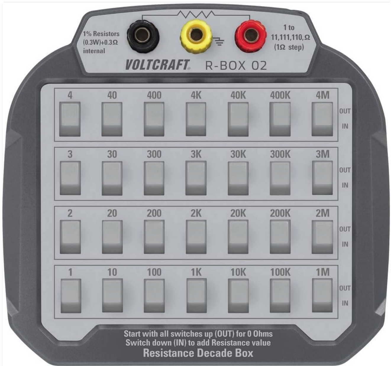
Figure 2: Close-up view of the VOLT CRAFT R-BOX 02. This image provides a clearer look at the individual switches and their corresponding resistance values, as well as the color-coded 4mm banana plug terminals (black, yellow, red) at the top for connecting to external circuits. The text on the device indicates "1% Resistors (0.3W) + 0.3Ω internal" and "1 to 11,111,110 Ω (1Ω step)".
