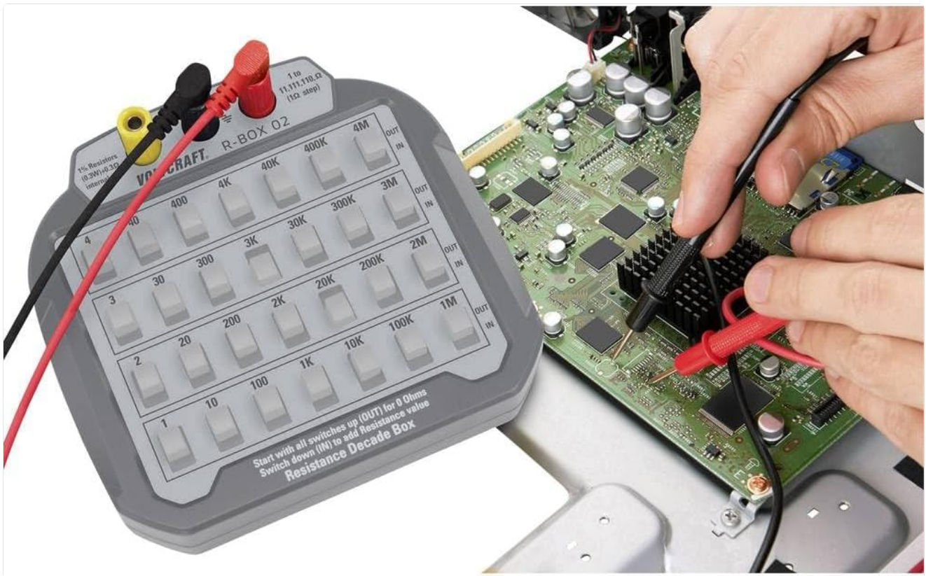
Figure 3: The VOLT-CRAFT R-BOX 02 connected to a circuit board. This image illustrates the decade box in an operational setting, with test leads connected from its 4mm terminals to a circuit board, demonstrating its application in electronic testing or development.
