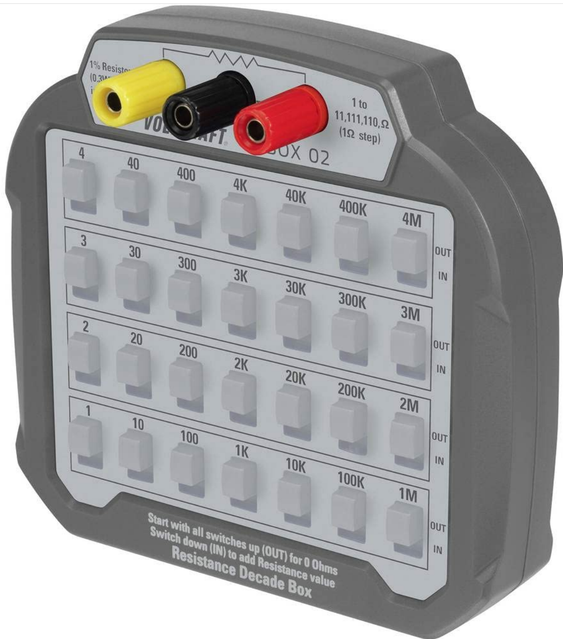
Figure 1: Front view of the VOLT CRAFT R-BOX 02. This image shows the main unit with its array of toggle switches, each labeled with resistance values, and the 4mm input/output terminals at the top. The labels indicate resistance ranges from 1 Ohm to 4M Ohm, with a note about 1% resistors and 0.3 Ohm internal resistance. Instructions at the bottom state "Start with all switches up (OUT) for 0 Ohms. Switch down (IN) to add Resistance value."
