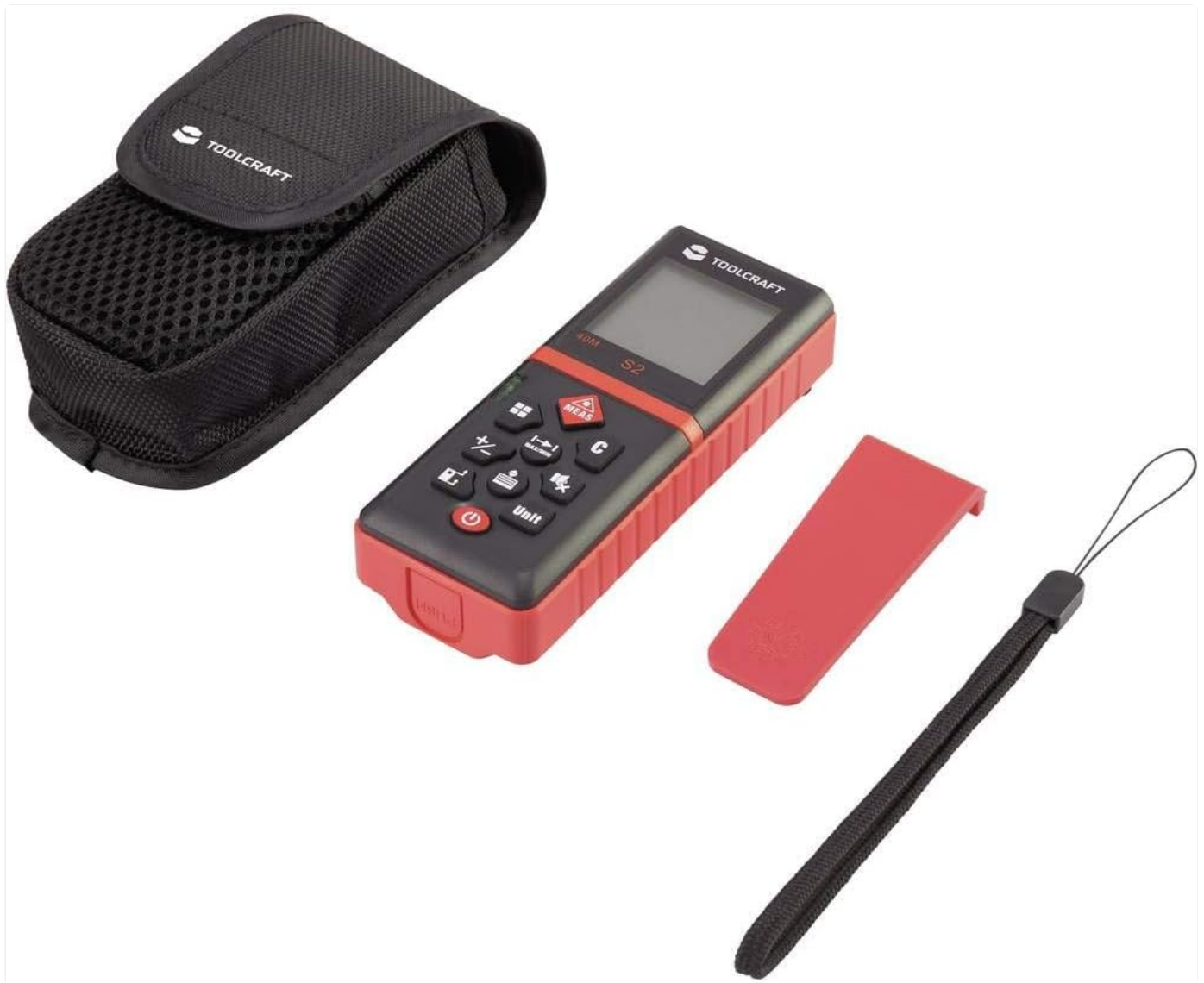
Figure 2: Contents of the TOOLCRAFT LDM X40 package, including the device, its protective pouch, and a wrist strap.
