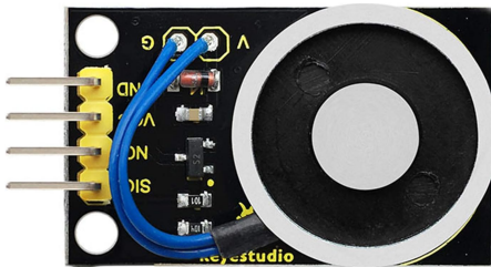
Figure 7.1: Top-down view of the KEYESTUDIO Electromagnet Module, showing the main components and connection pins.
