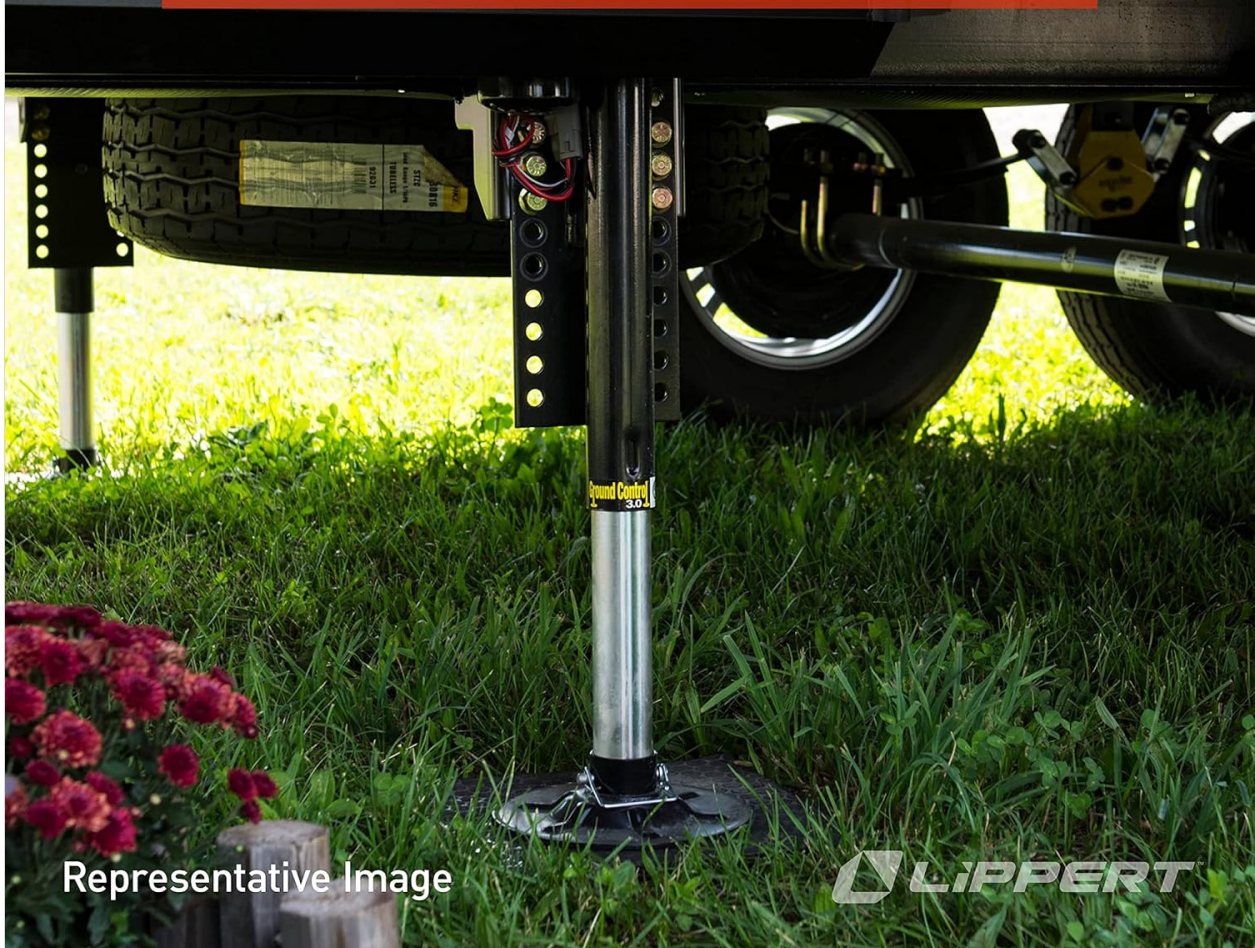
Figure 5.1: An RV leveling jack extended during the automatic leveling process.
