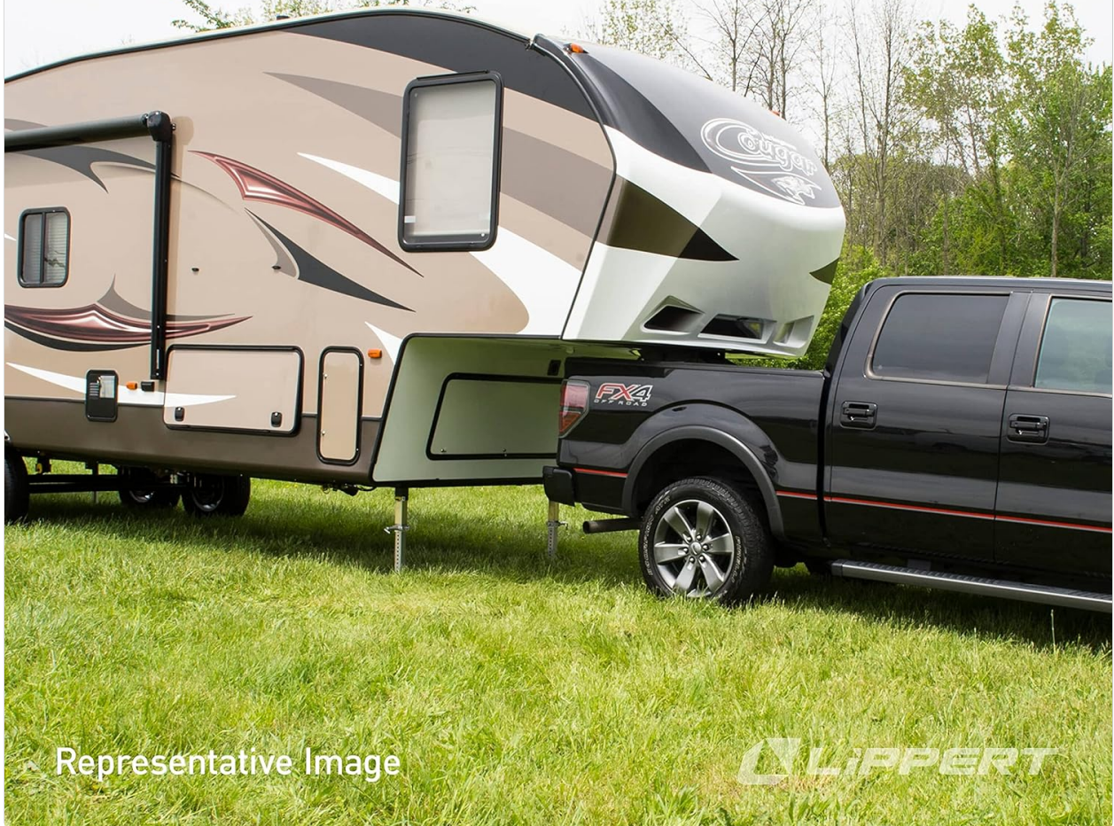
Figure 5.2: An RV prepared for re-hitching using the auto-hitch memory feature.
