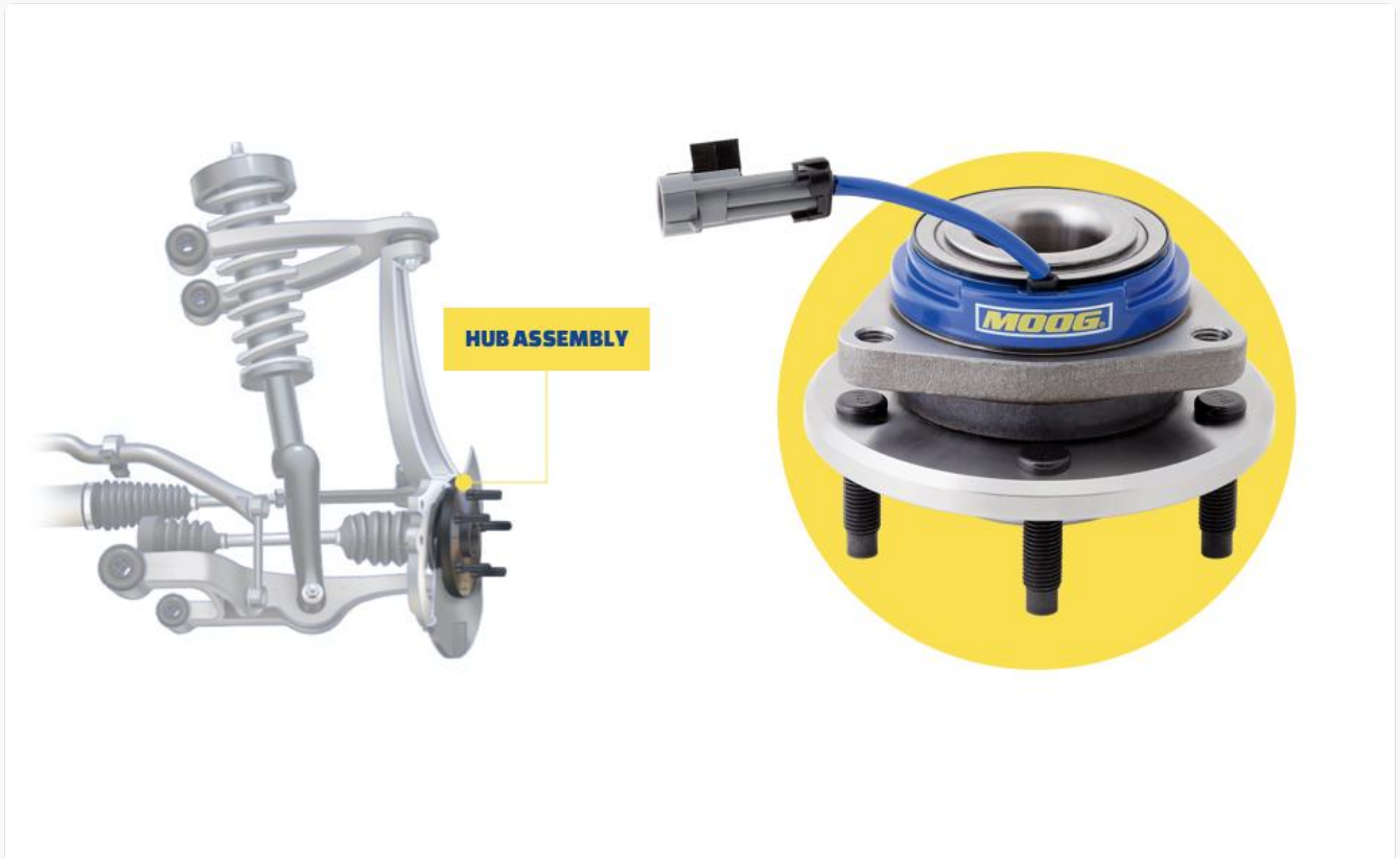
Figure 6: Illustration of a hub assembly's location within a vehicle's suspension system.
