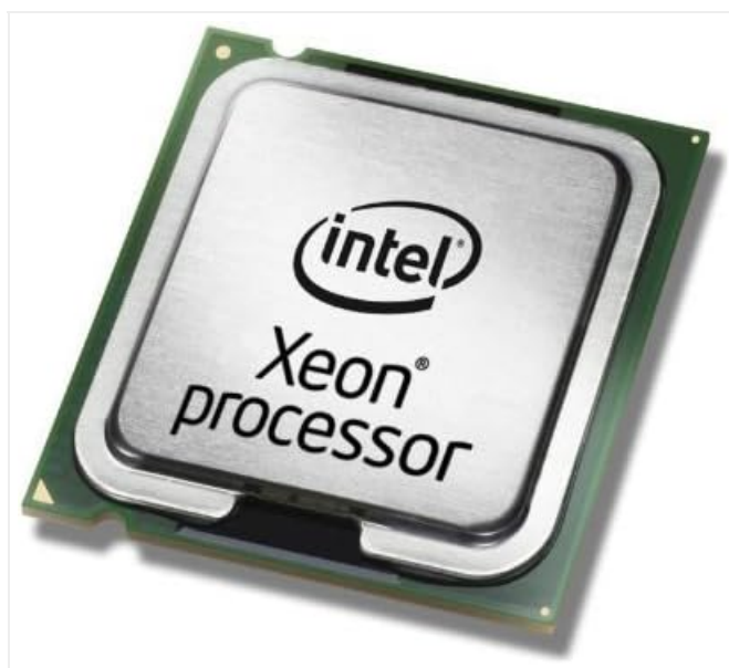
Figure 2.1: Top view of the Intel Xeon E5-2670 processor, showing the integrated heat spreader with Intel branding.
