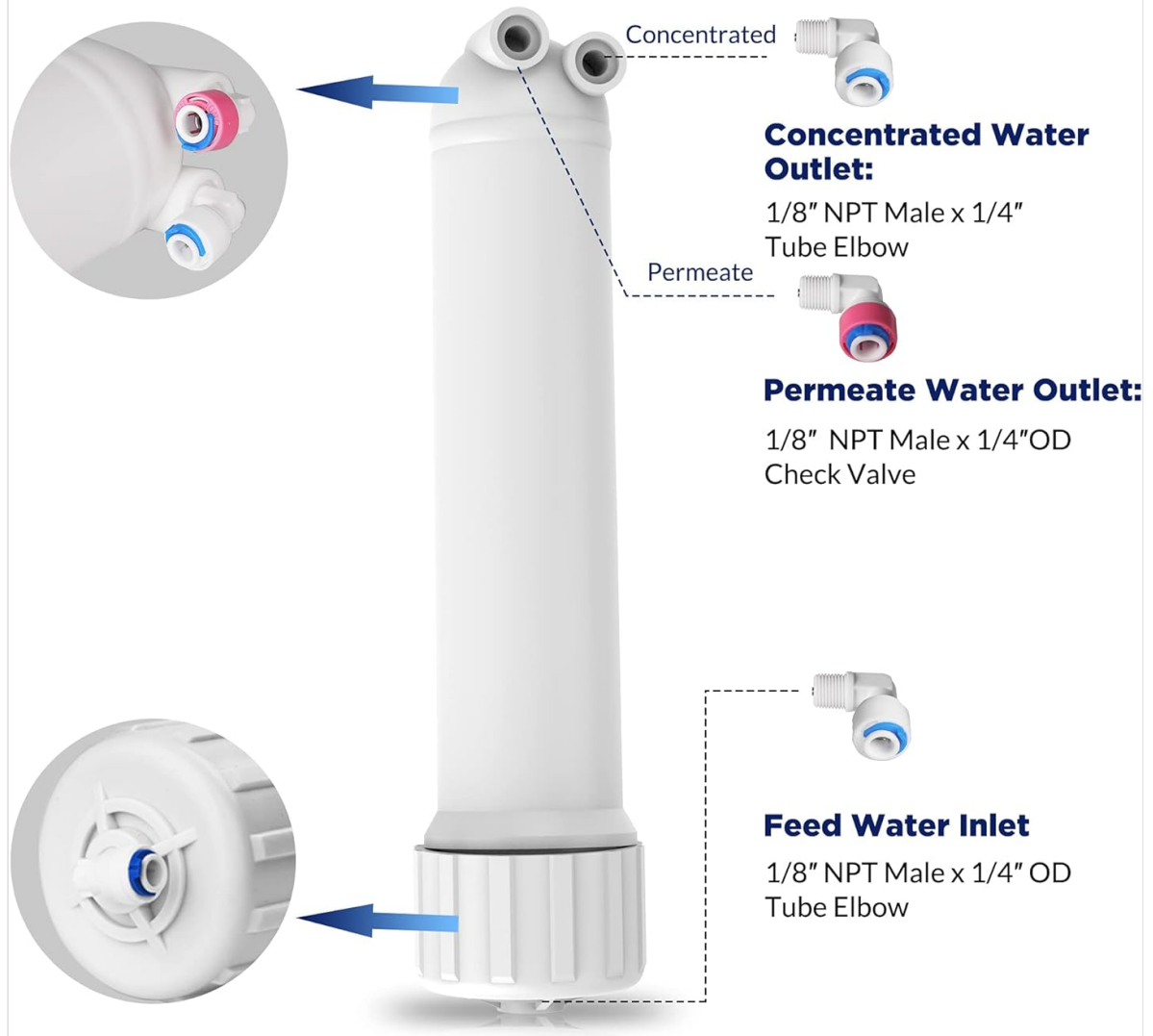
Figure 4: The easy installation kit includes standard screwed fittings for simple setup. Ensure correct connections for feed water, permeate, and concentrated water.
