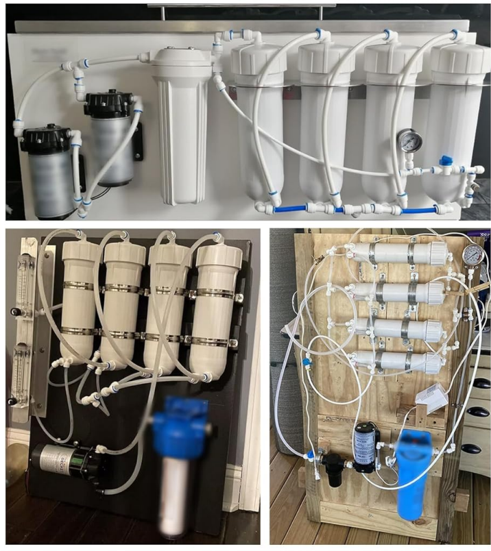
Figure 7: DIY RO systems, like those using this membrane, can be used for concentrating maple sap, significantly reducing boil time.
