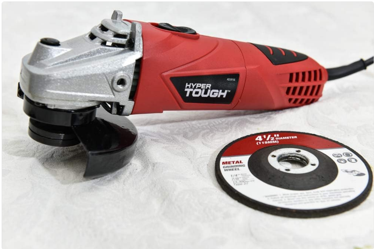
Figure 3.3: The Hyper Tough angle grinder with a 4 1/2 inch grinding wheel properly installed and the adjustable guard in position.
