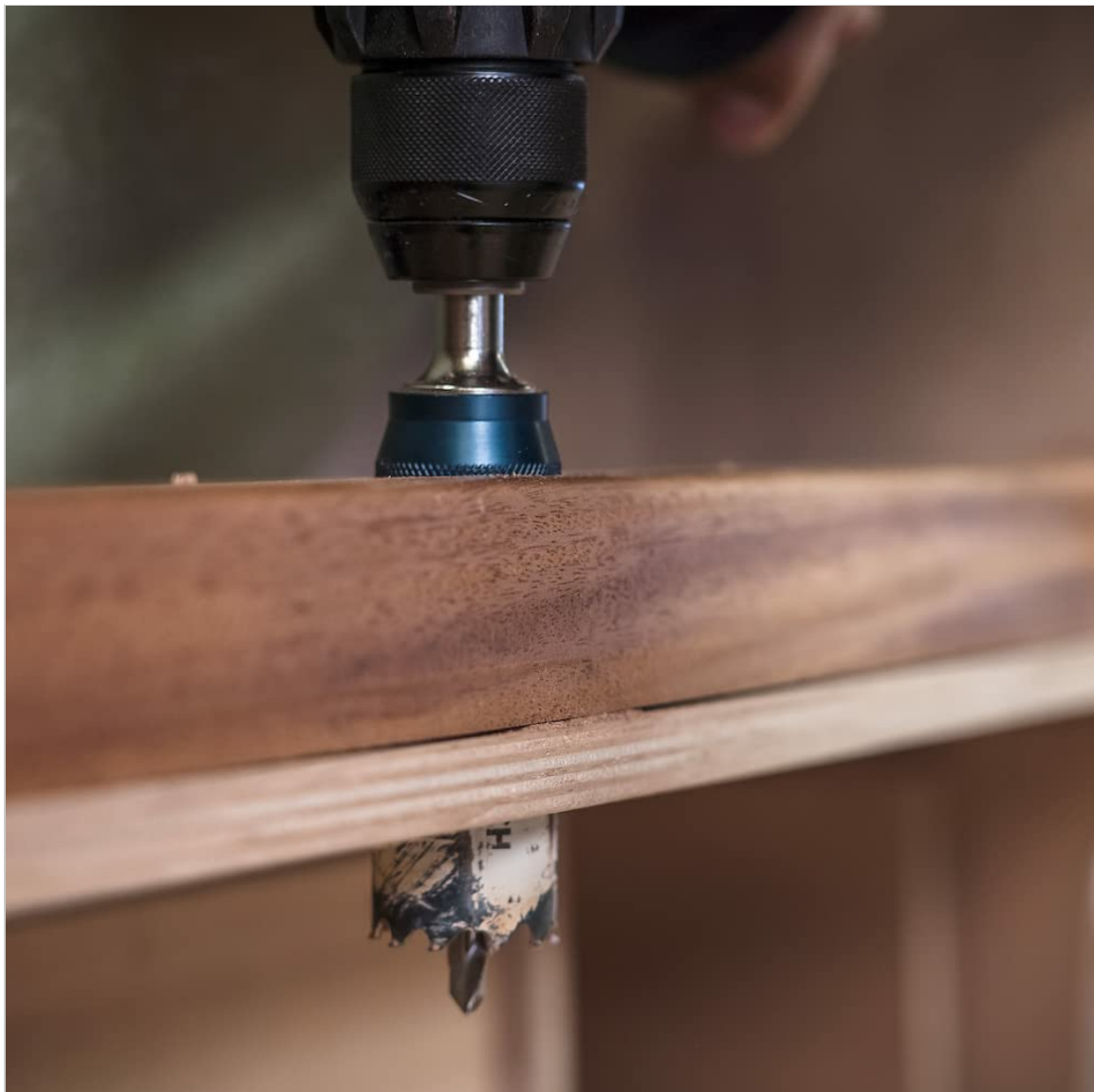
Figure 5.3: Illustrates the adapter and hole saw completing a cut from the underside of a wooden surface.
