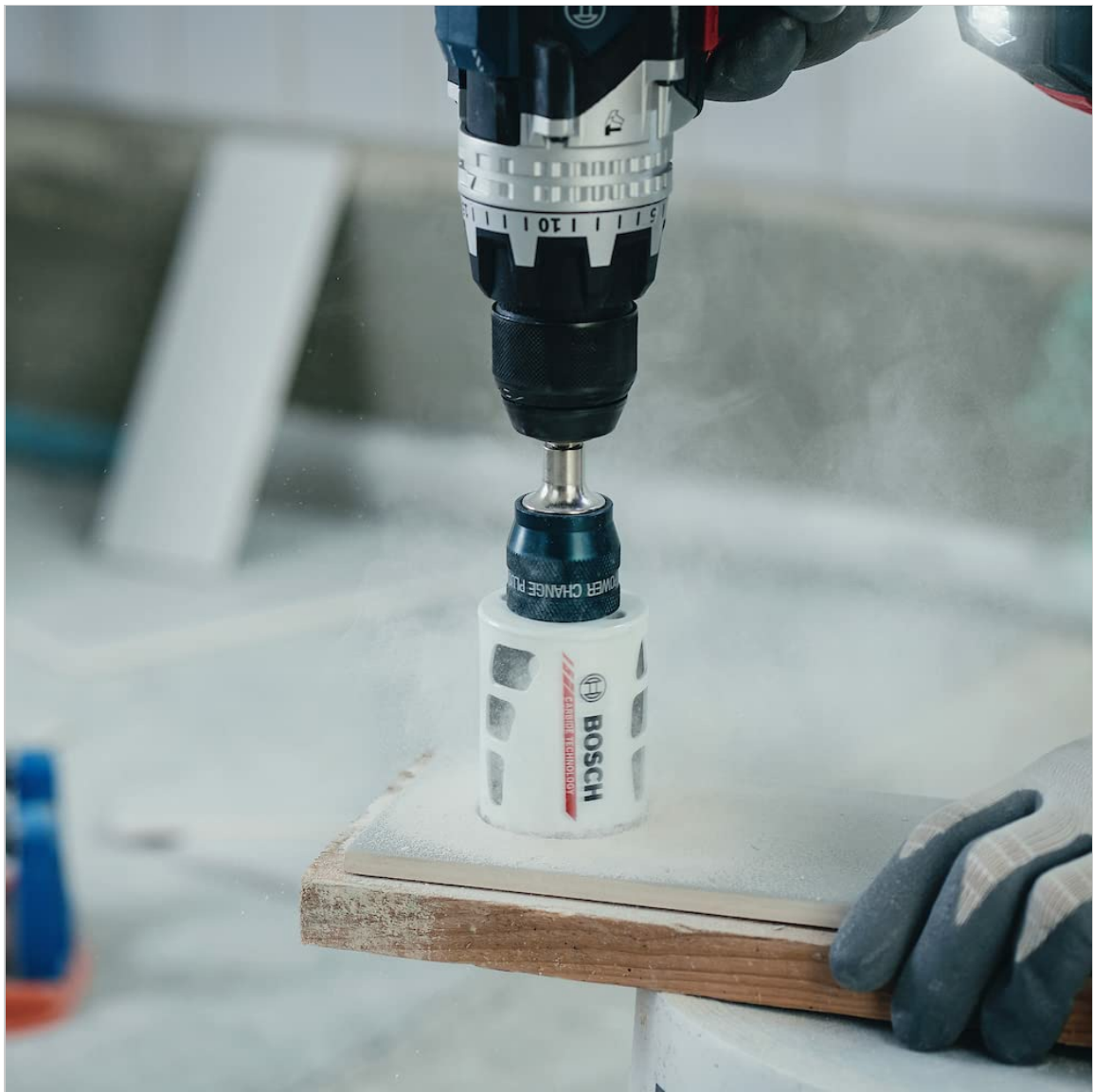
Figure 5.2: The adapter and hole saw effectively cutting a clean hole in a wooden board.
