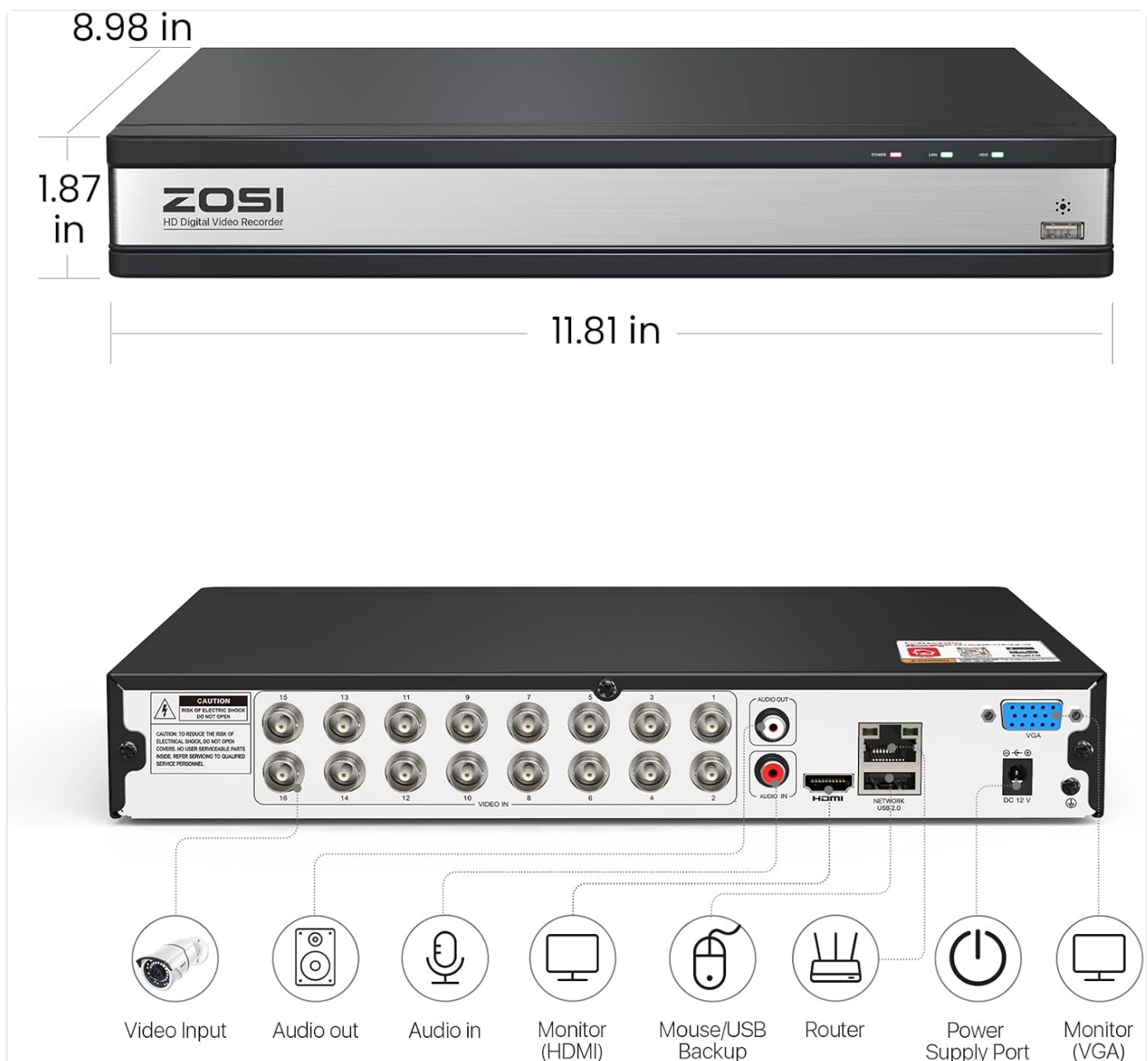
Image: A diagram detailing the physical dimensions of the ZOSI DVR unit and an annotated view of its rear panel. Key connectors shown include 16 BNC video input ports, RCA audio input and output, HDMI and VGA ports for monitor connection, an Ethernet port for network connectivity, a USB port for mouse and backup devices, and the DC 12V power input.
