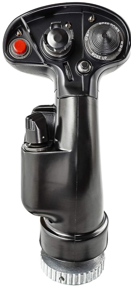
Top view of the F/A-18 Grip, showing the hat switches and primary buttons.
