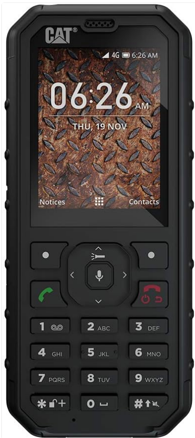
Front View: Displays the screen, navigation buttons, and alphanumeric keypad.
