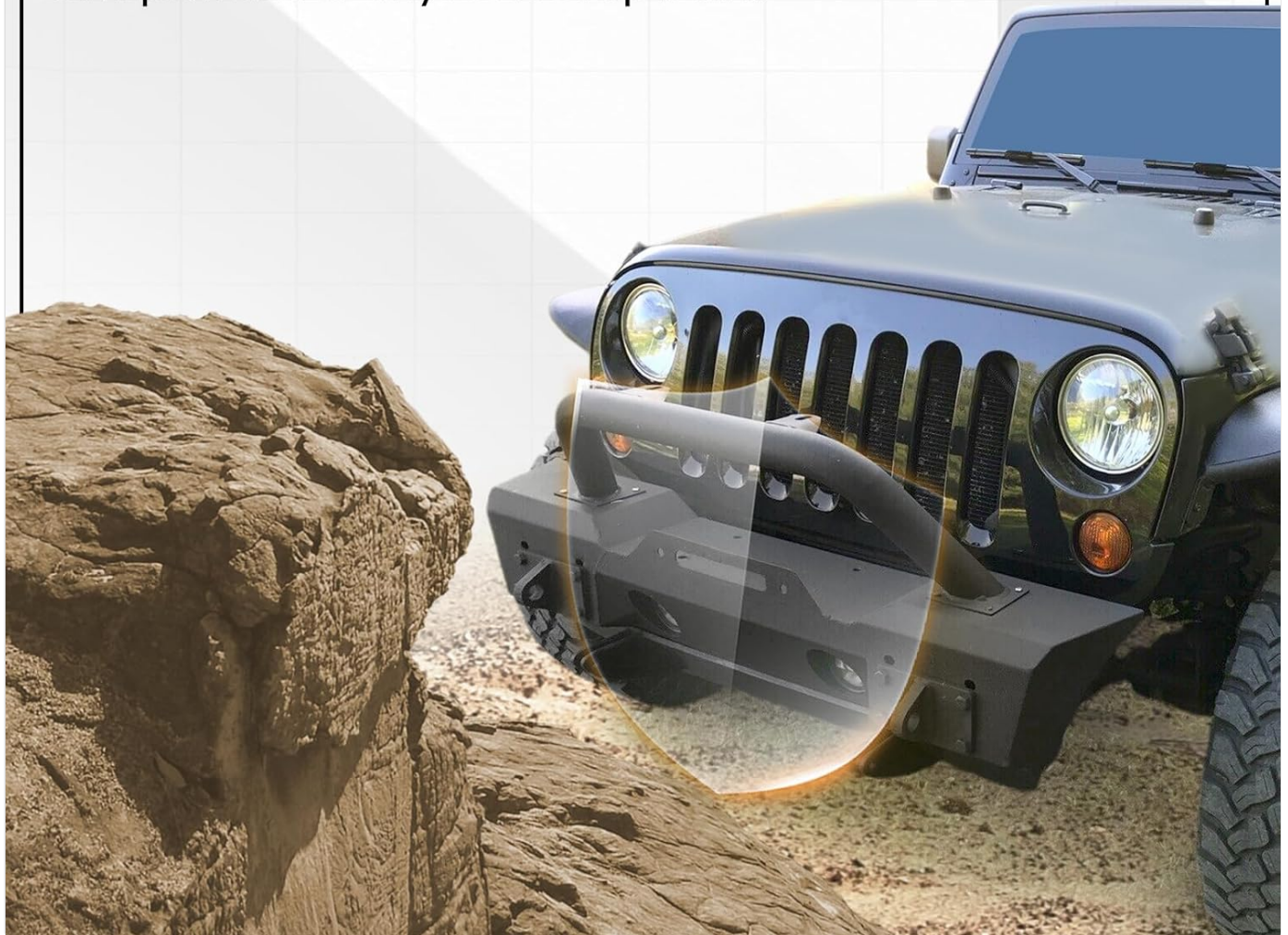
Figure 3.2: The stubby design provides improved approach angles for off-road use.
