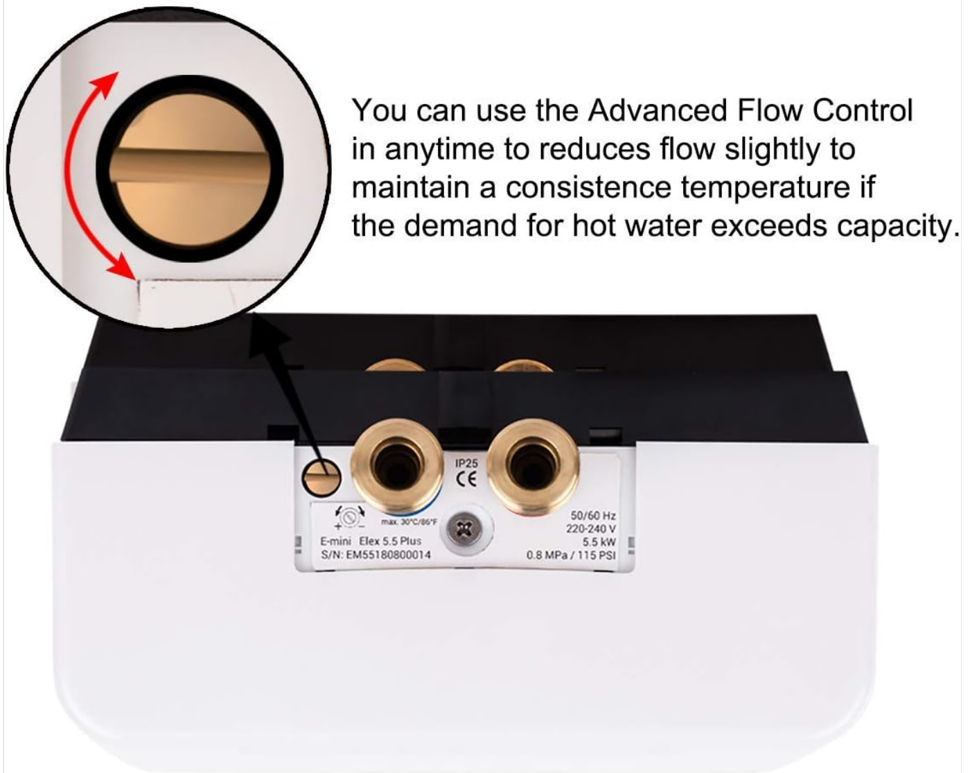
Figure 6.1: Detail of the Advanced Flow Control mechanism, which can be adjusted to slightly reduce flow and maintain consistent temperature if hot water demand exceeds the unit's capacity.
