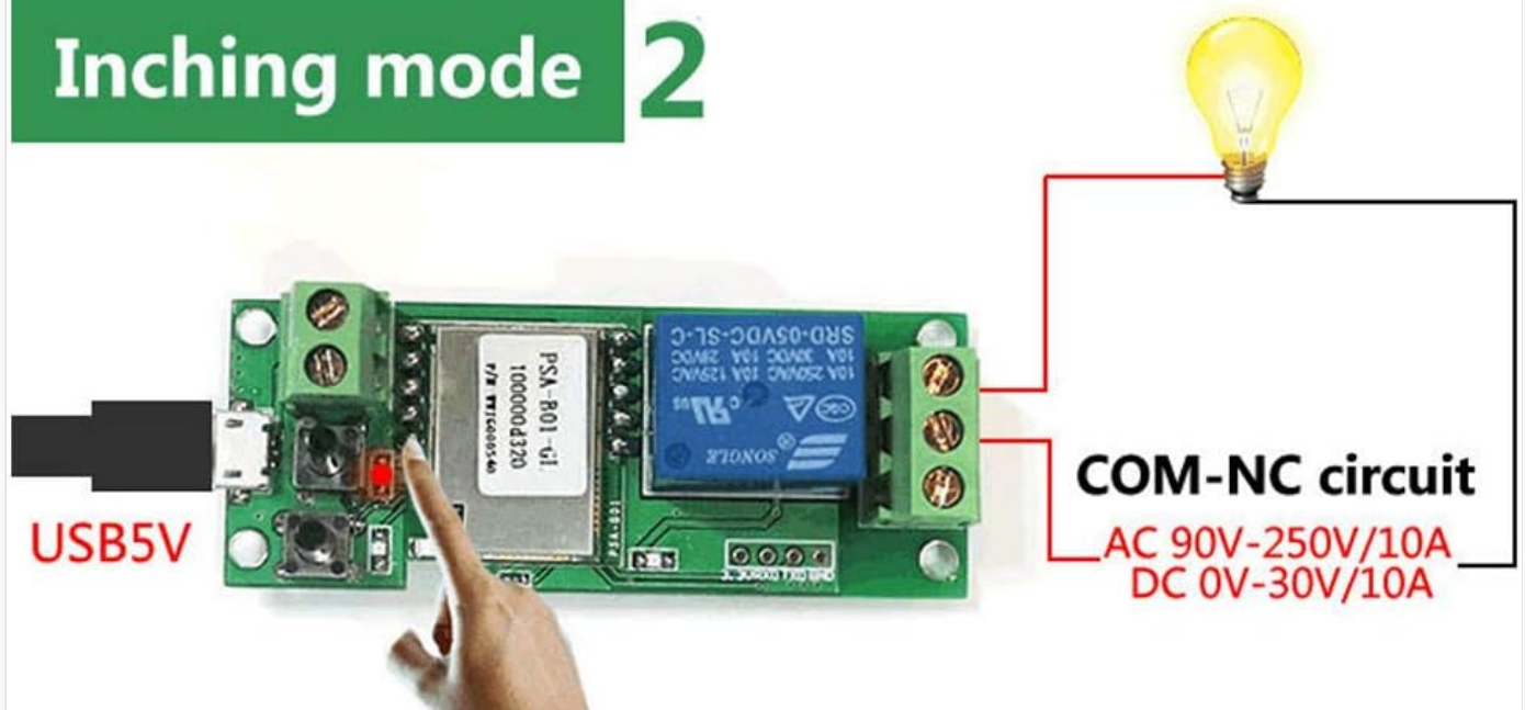
Image 5.1: Visual representation of Inching Mode. The top diagram shows a COM-NO circuit, where a brief activation turns on a light. The bottom diagram shows a COM-NC circuit, where a brief activation turns off a light.
