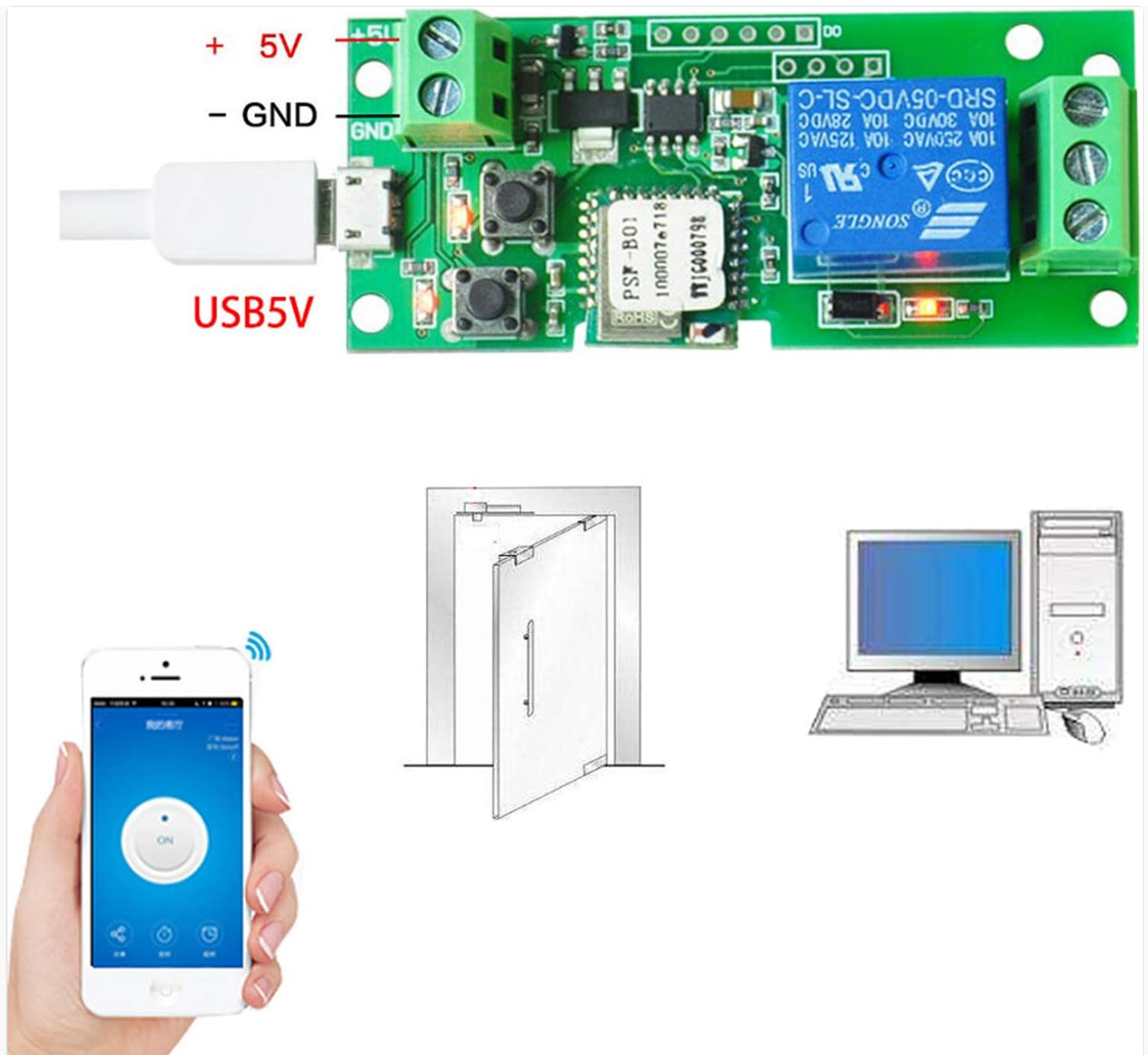
Image 4.1: The smart switch module powered via a USB 5V cable, illustrating the connection to the USB port and the alternative 5V/GND screw terminals.
