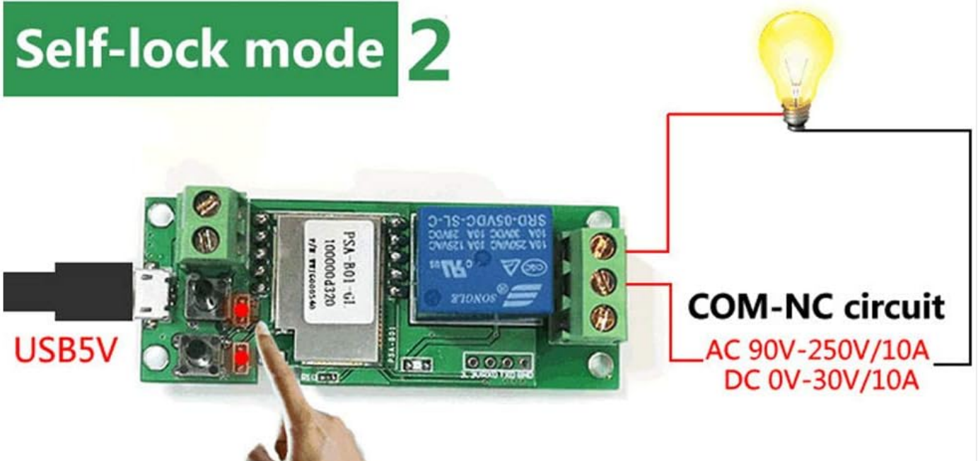
Image 5.2: Visual representation of Self-Locking Mode. The top diagram shows a COM-NO circuit, where activation switches the light on/off. The bottom diagram shows a COM-NC circuit, where activation switches the light off/on.
