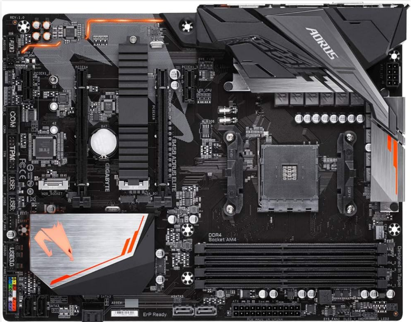
Image 3.1: Top-down view highlighting key component locations on the motherboard, including CPU socket, DIMM slots, and PCIe slots.
