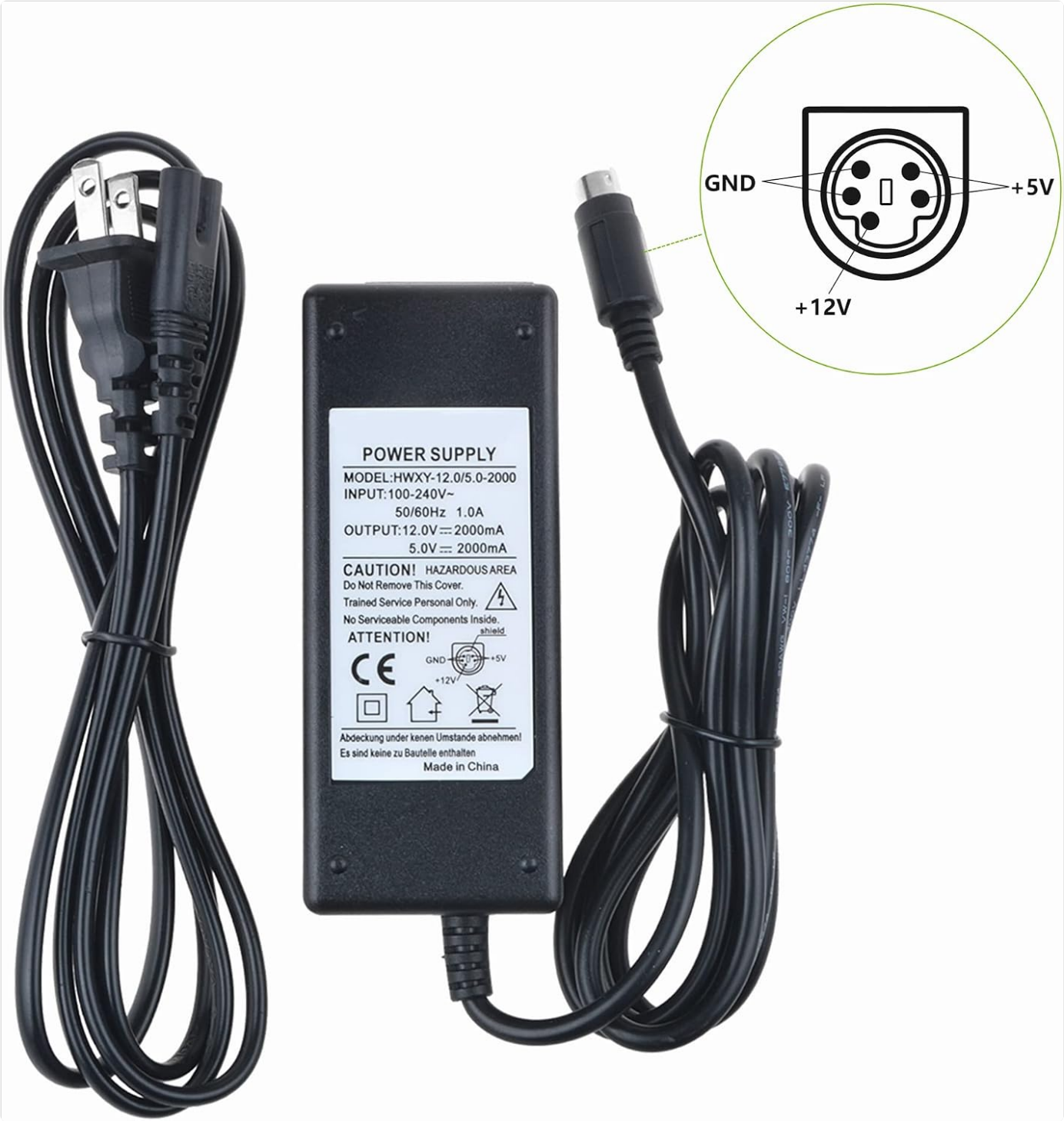
Image 5.1: The power supply unit, displaying its model and input/output specifications, alongside a diagram detailing the pinout of the round connector (GND, +5V, +12V).
