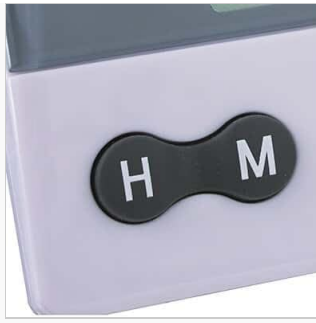
Image: Close-up of the 'H' (Hours) and 'M' (Minutes) buttons, which are used for setting time values.
