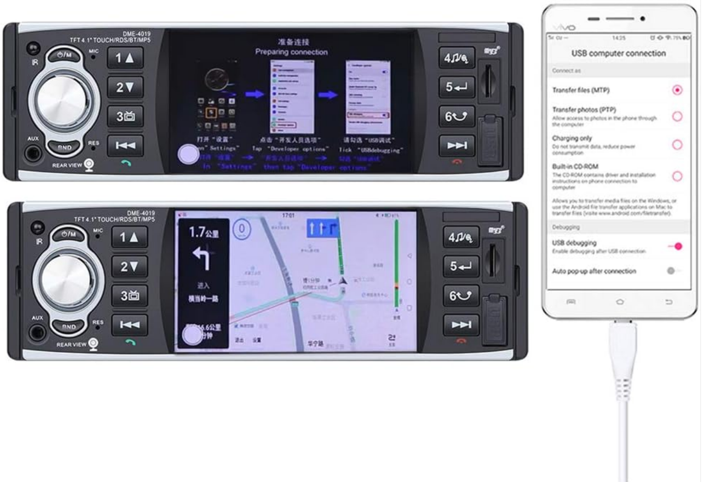
Image 3.6: Diagram illustrating the Mirror Link connection process for Android phones, showing the phone screen mirrored on the car MP5 player's display.
