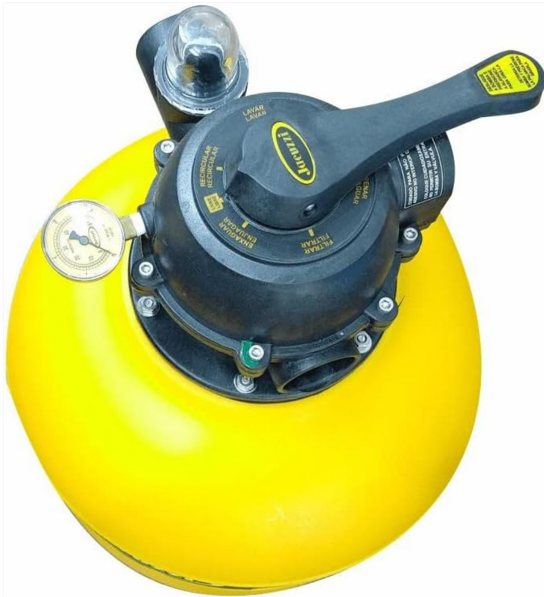
Figure 2.1: A close-up top view of the filter's multi-port valve, showing the handle, pressure gauge, and various operational settings.
