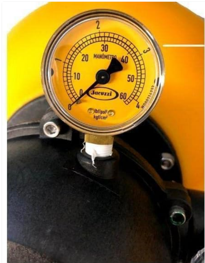
Figure 4.1: Detailed view of the pressure gauge, indicating filter pressure in PSI and kgf/cm².
