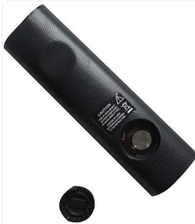
Figure 2: Remote control showing the battery cap detached.
