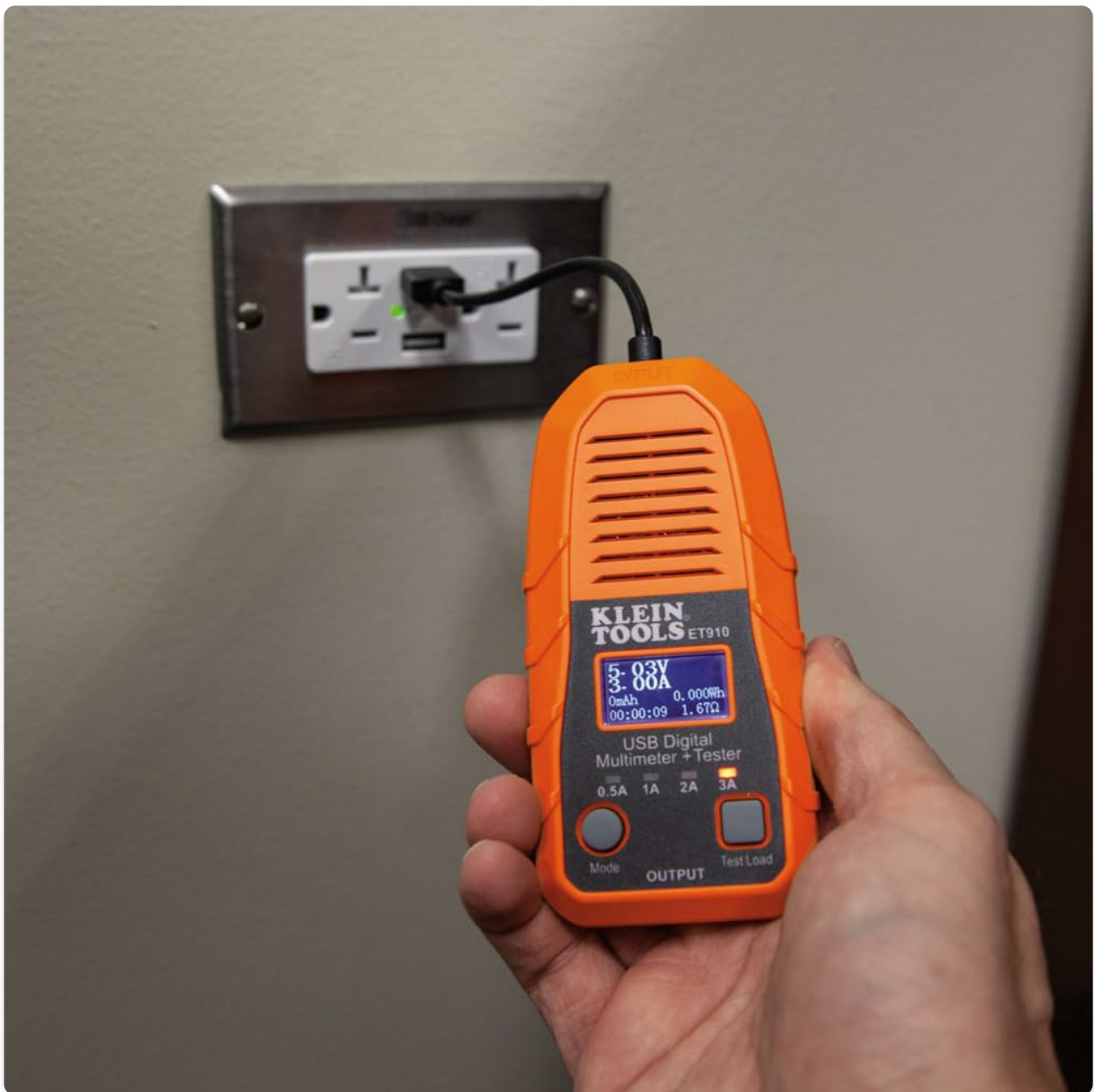
Figure 3: The ET910 in monitoring mode, showing its display while connected to a wall charger. The screen provides clear, real-time data.
