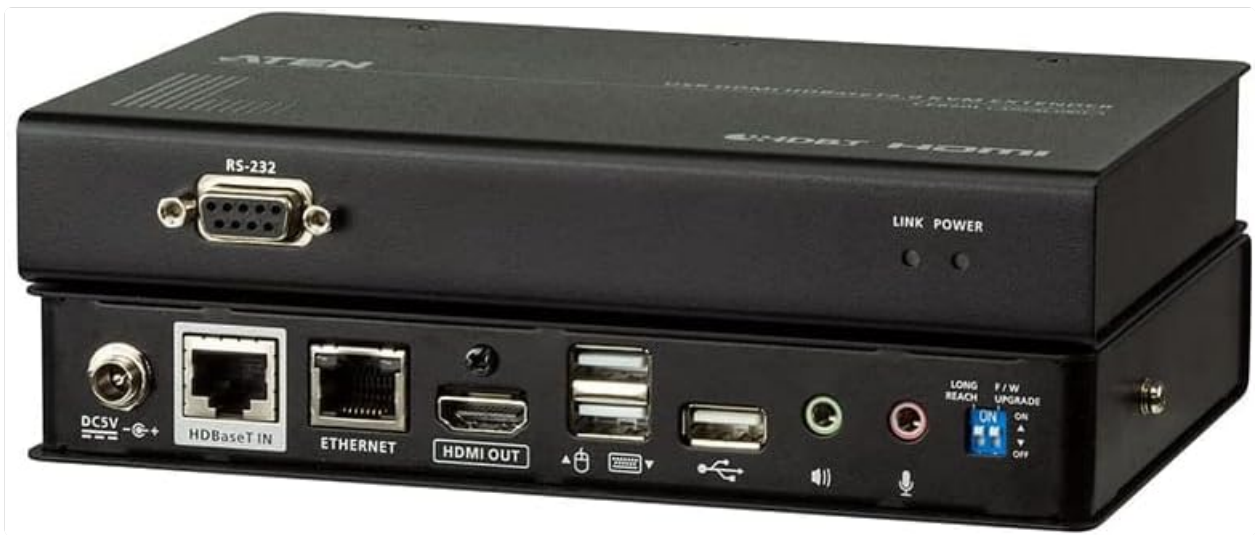
Image 3.1: Rear view of the ATEN CE820 KVM Extender units, showing various ports including DC power, HDBaseT In/Out, Ethernet, HDMI, USB, audio jacks, RS-232, and DIP switches for mode selection.
