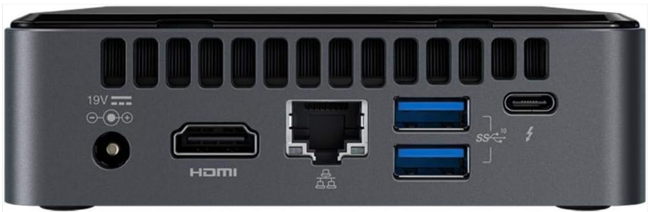
Figure 3: Detailed view of the rear panel. This panel features the DC power input (19V), an HDMI port, a Gigabit Ethernet port, two additional USB 3.1 Gen2 Type-A ports, and a USB-C port with Thunderbolt 3 capabilities.
