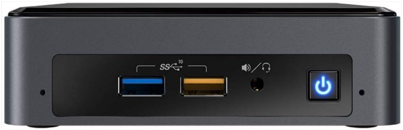
Figure 2: Detailed view of the front panel. It includes two USB 3.1 Gen2 Type-A ports (one yellow for charging), a 3.5mm audio jack (headphone/microphone combo), and the power button with an LED indicator. A small SD card slot is also visible on the side.
