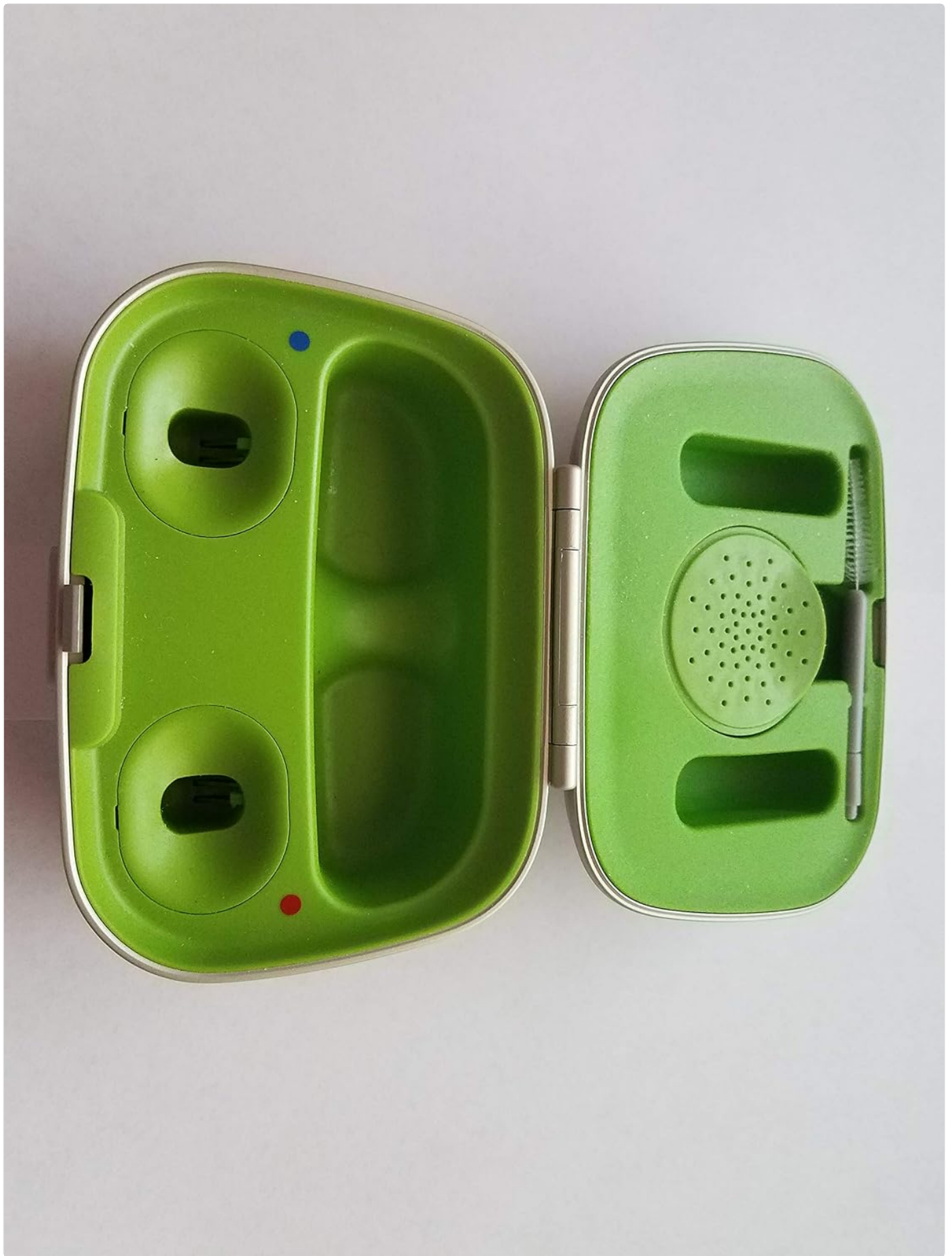
Figure 2: Interior view of the open Phonak Charger Case RIC, displaying the two hearing aid charging slots (left and right, indicated by blue and red dots respectively) and the integrated cleaning tool compartment on the right.
