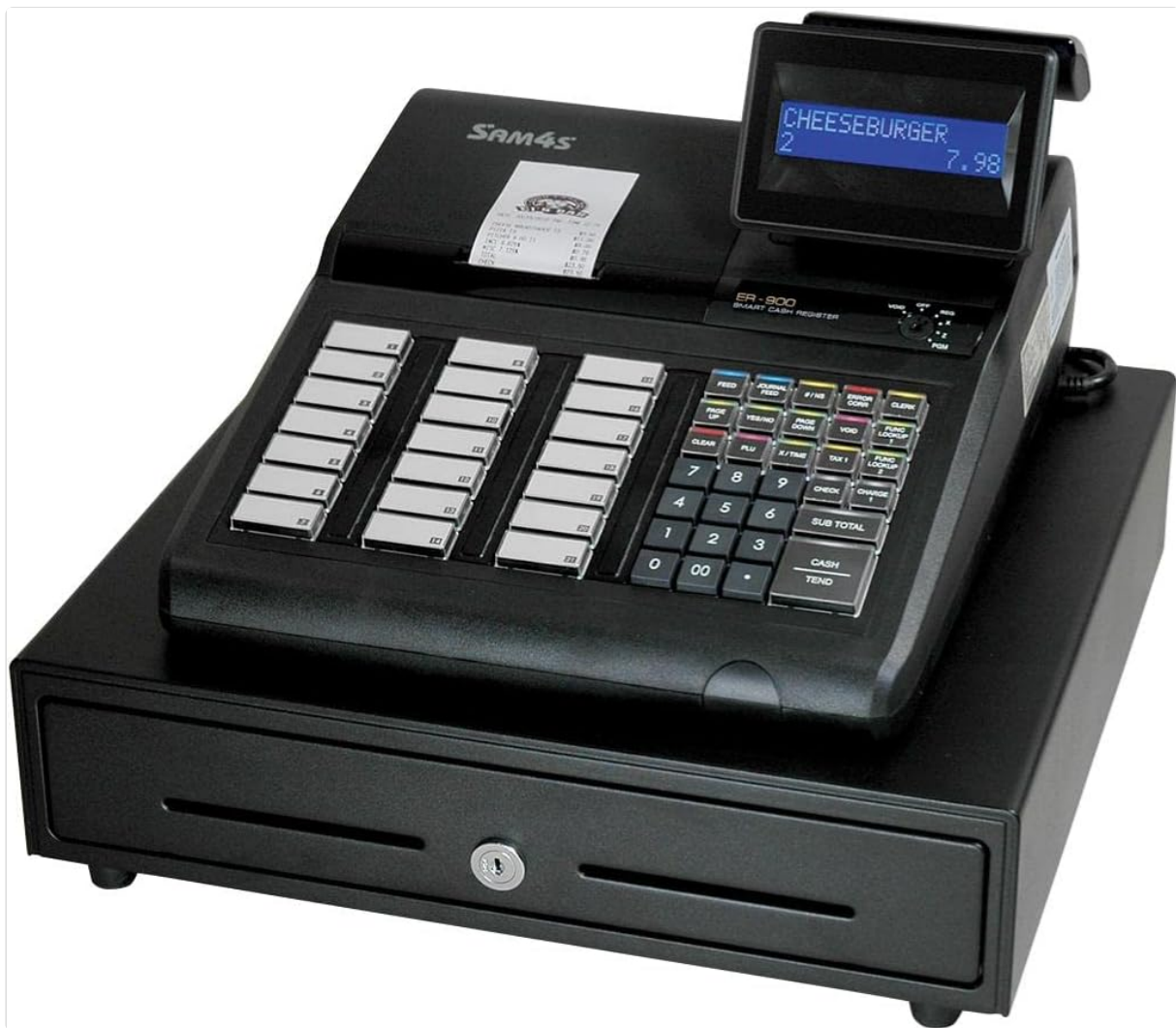
Figure 1: SAM4s ER-925 Cash Register with Metrologic Fusion Barcode Scanner. The image shows the main unit with a display showing "CHEESEBURGER 2 7.98", a receipt printer, a numeric keypad, function keys, and a cash drawer below.
