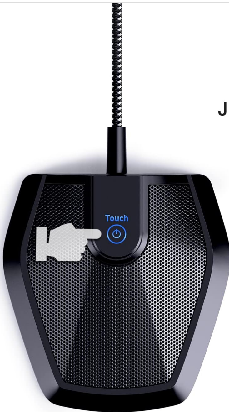
Figure 5.1: The touch-sensitive mute button on the TONOR G11 microphone. A blue light indicates active recording, while a different state (e.g., off) indicates mute.
