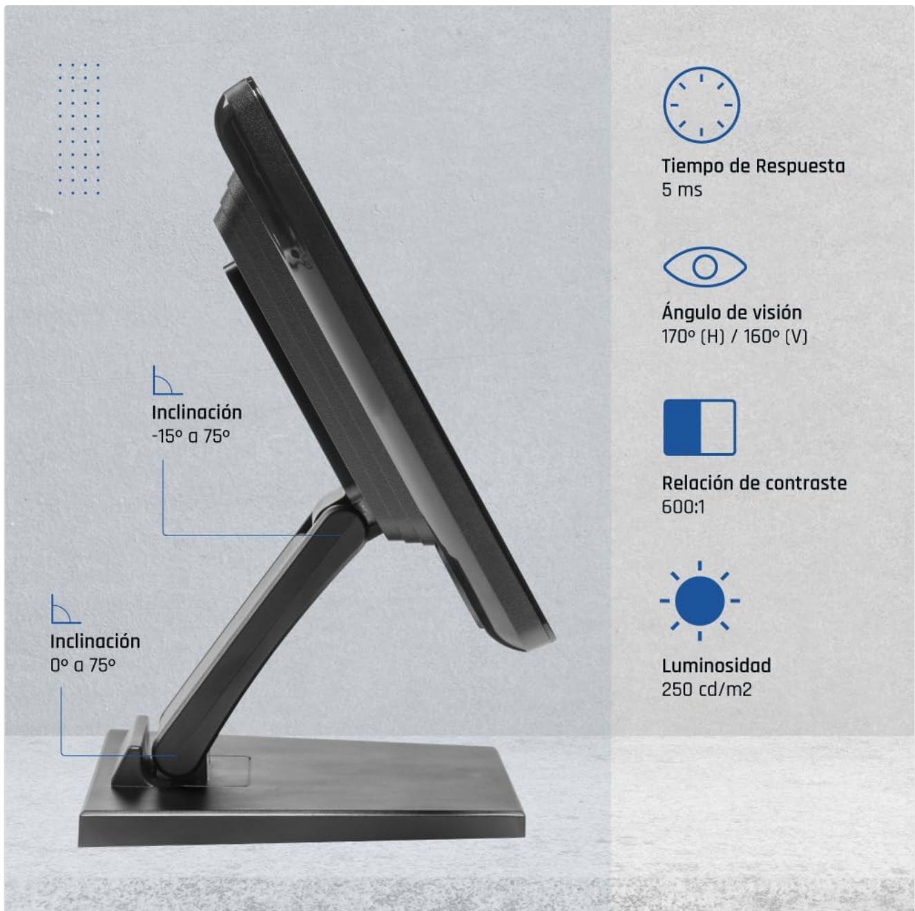
Image 5.3: Diagram illustrating the adjustable tilt range of the monitor, from -15 degrees to 75 degrees.
