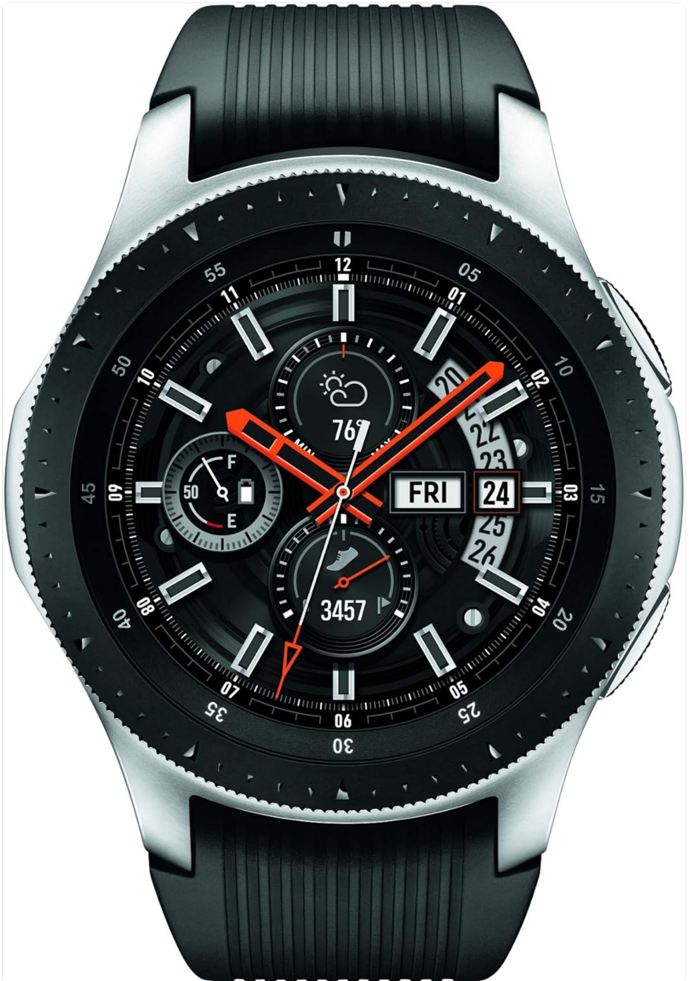
Figure 1: Front view of the Samsung Galaxy Watch 46mm. This image shows the watch's circular display, rotating bezel, and the standard black silicone strap. The watch face displays digital time, date, and weather icons, along with activity tracking elements.
