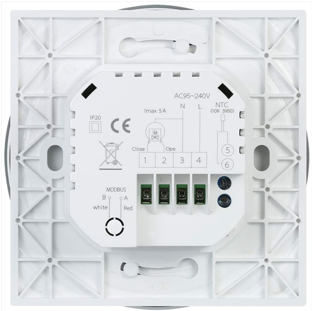
Figure 5: Detailed wiring diagram for the Decdeal WiFi Thermostat, showing connections for AC power (N, L), load (1, 2), and NTC sensor (5, 6).
