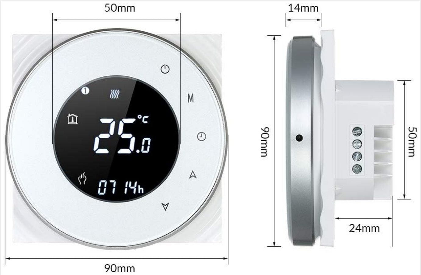
Figure 4: Dimensional drawing of the Decdeal WiFi Thermostat, showing front and side measurements.
