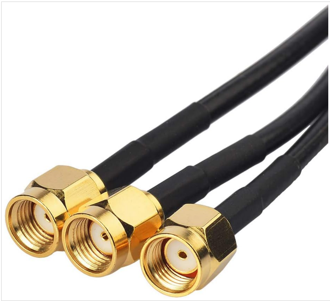
Image: Close-up view of the three RP-SMA male connectors on the antenna cable. Note the internal threads and absence of a center pin, which is characteristic of RP-SMA male connectors.
