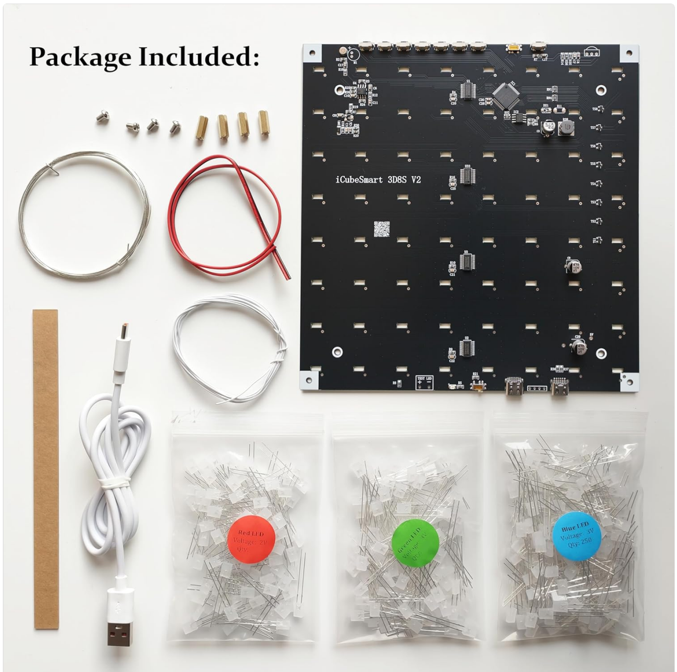
Figure 2: All components included in the iCubeSmart 3D LED Cube DIY kit, laid out for inspection.
