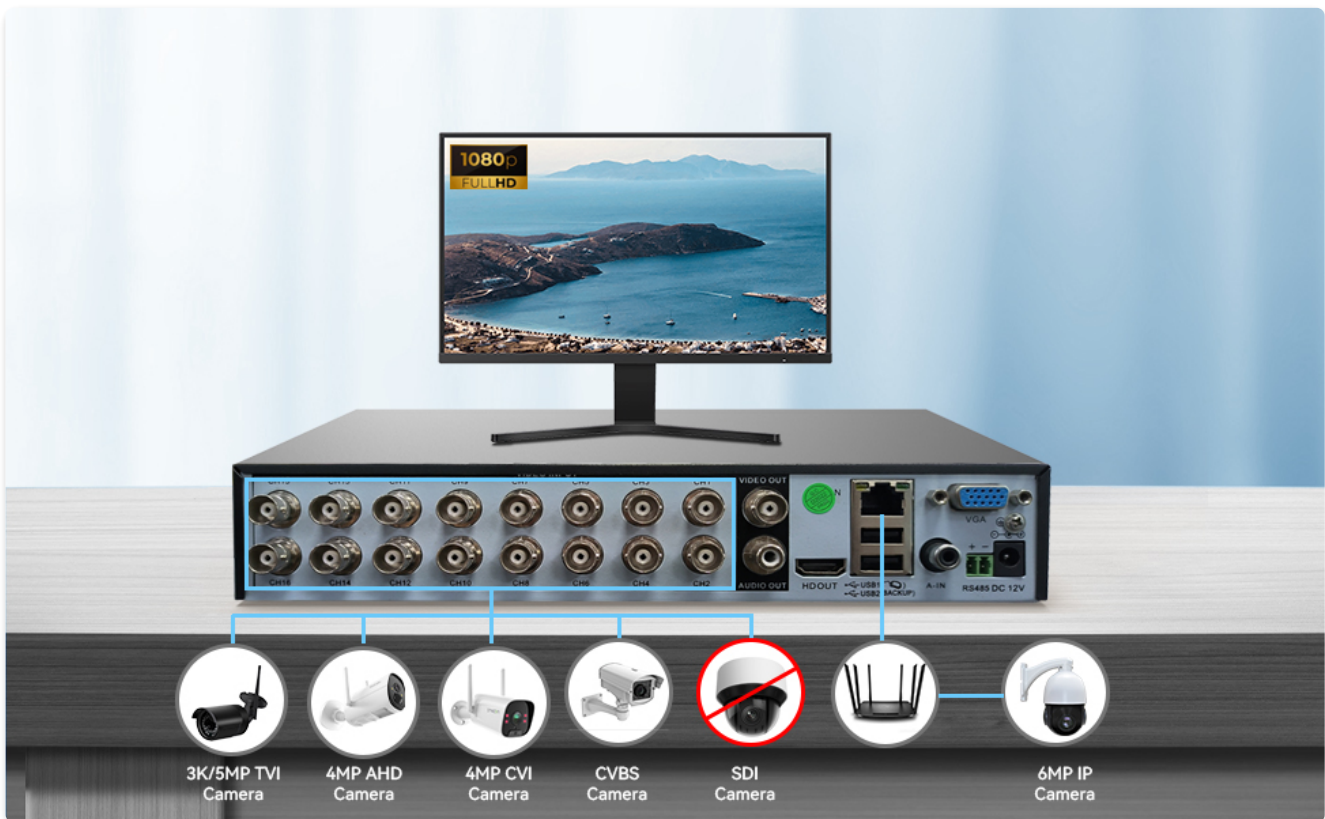
Figure 2.3: Illustration of the DVR's 5-in-1 compatibility, showing connections for 3K/5MP TVI, 4MP AHD, 4MP CVI, CVBS, and 6MP IP cameras. SDI cameras are not compatible.
