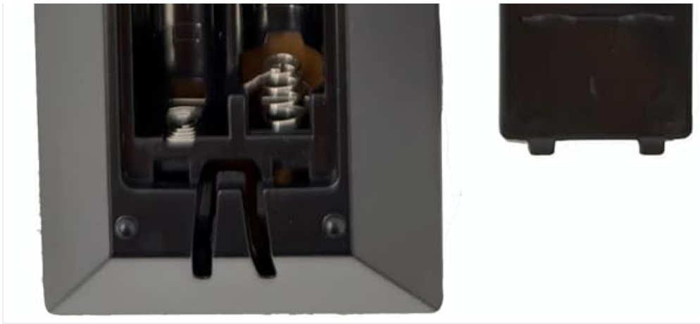
Figure 2: Rear view of the Smartby RMT-TX100U remote control, illustrating the open battery compartment and the correct orientation for AAA battery insertion.
