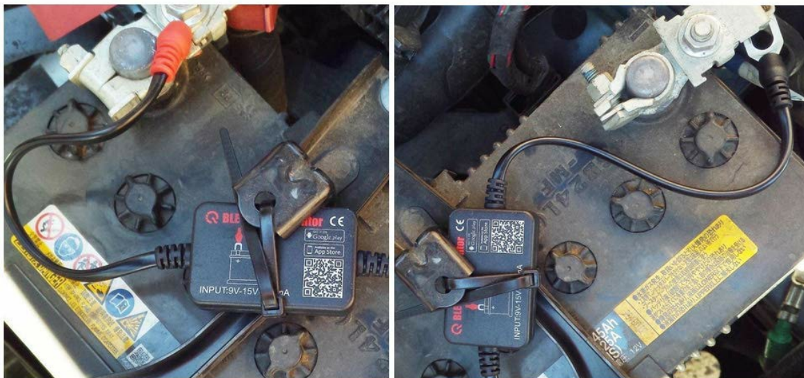
Figure 3: Proper installation of the battery monitor leads to the positive and negative terminals of a car battery.
