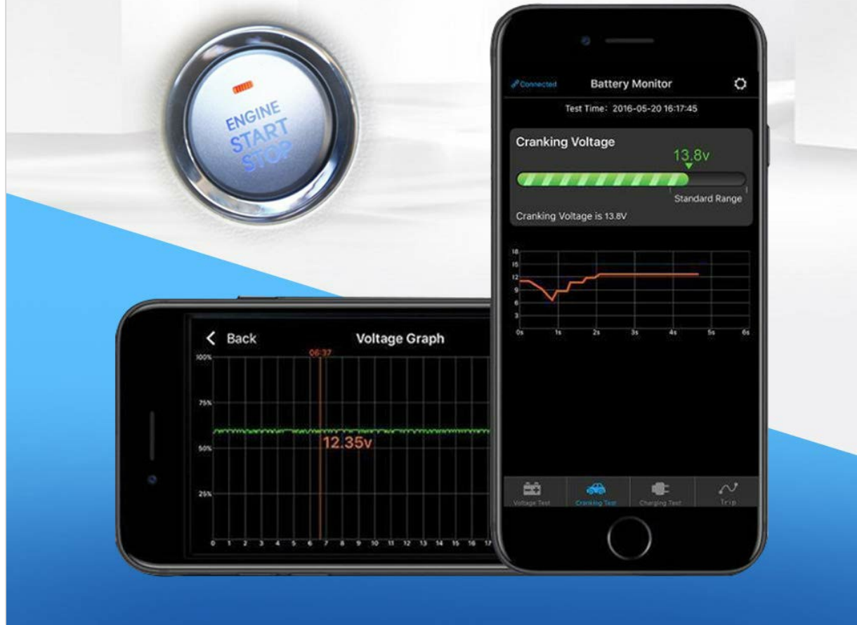
Figure 6: App display for the cranking test, showing cranking voltage and status.
