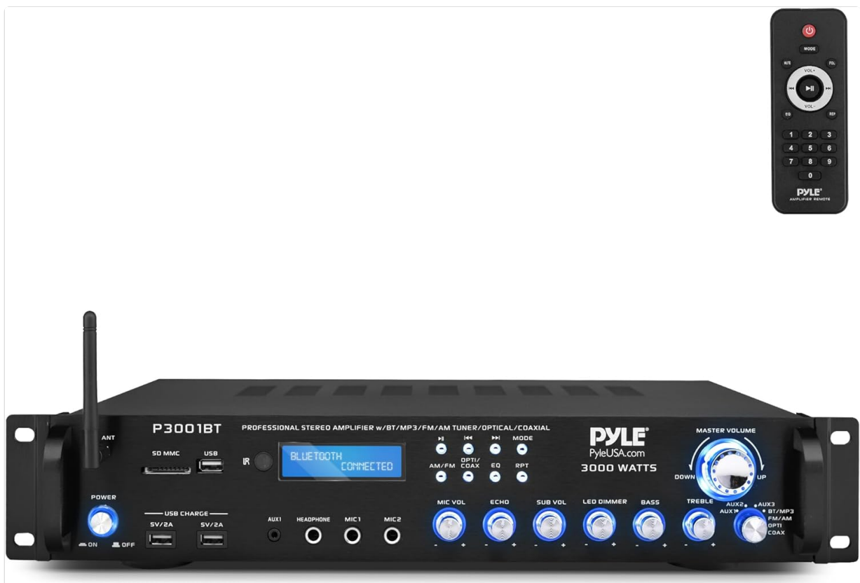
Image 4.1: Front view of the Pyle P3001BT amplifier, showing the power switch, USB/SD slots, Bluetooth display, input selectors, microphone inputs, and various control knobs.
