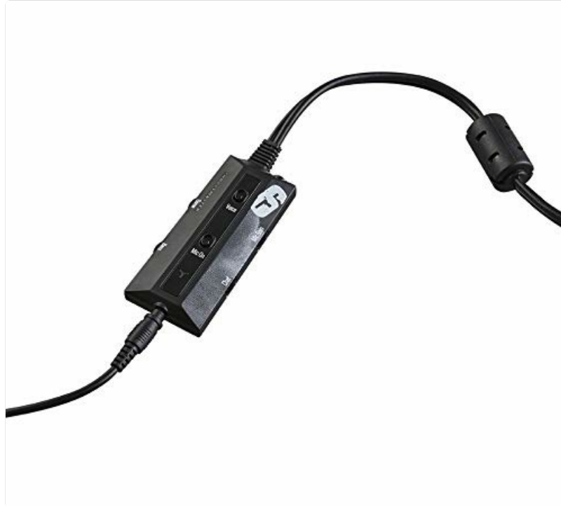
Figure 2: In-line control unit for volume and microphone adjustments.
