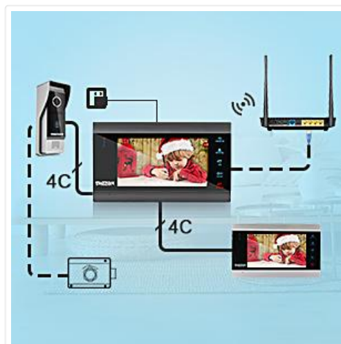
Figure 3.2: System Connection Diagram. This diagram illustrates how the 4-core cable integrates various components into a complete security and communication system.
