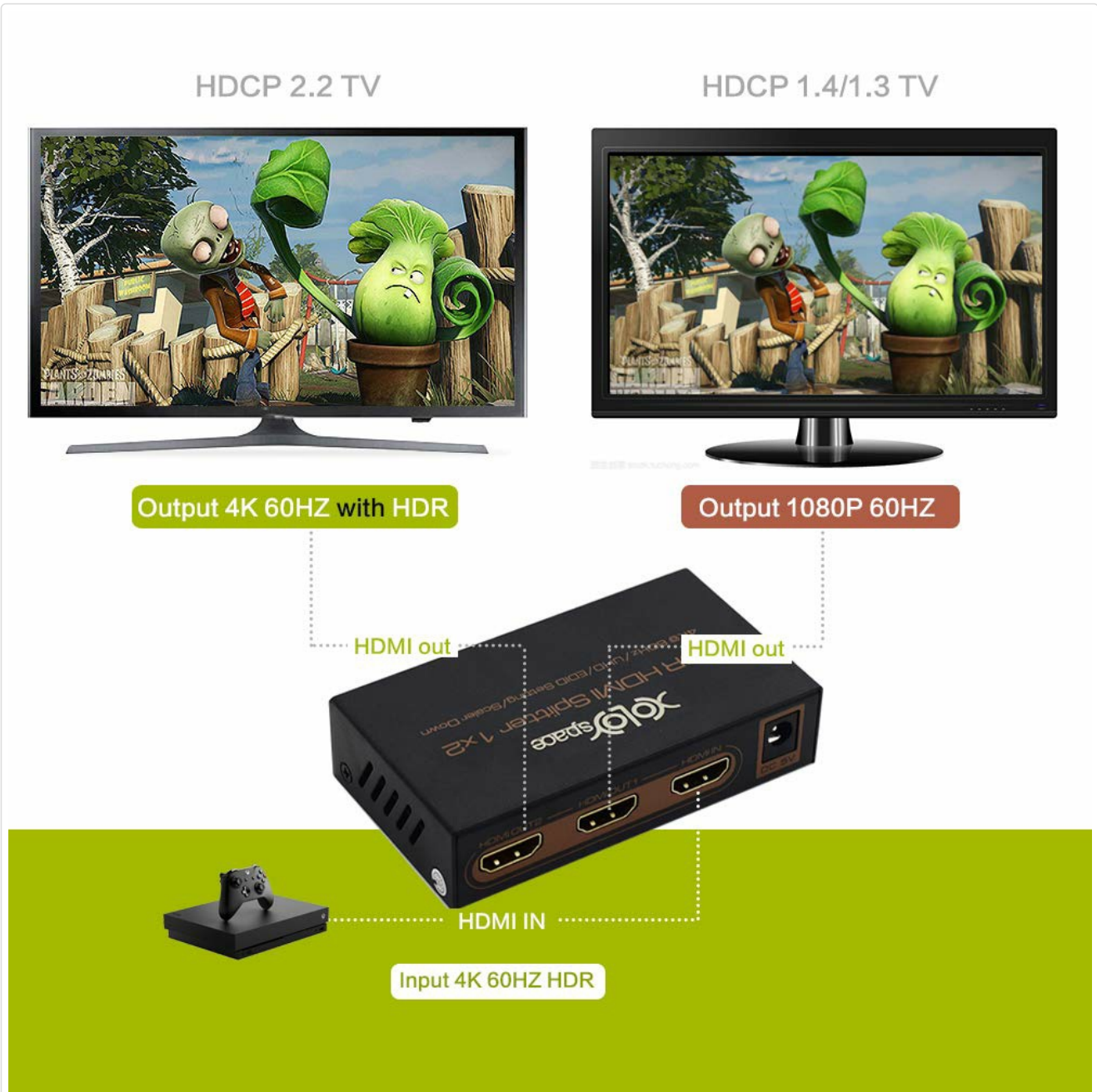
Figure 3: Automatic Downscaling Example. A 4K 60Hz HDR input is split, with one output remaining 4K 60Hz HDR for a compatible TV, and the other output downscaled to 1080p 60Hz for an older TV.
