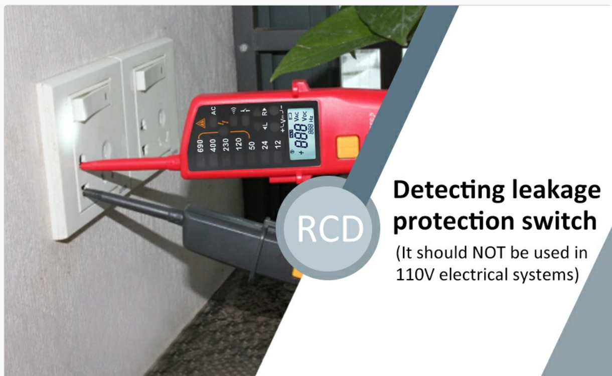
Figure 5: Performing an RCD test.
