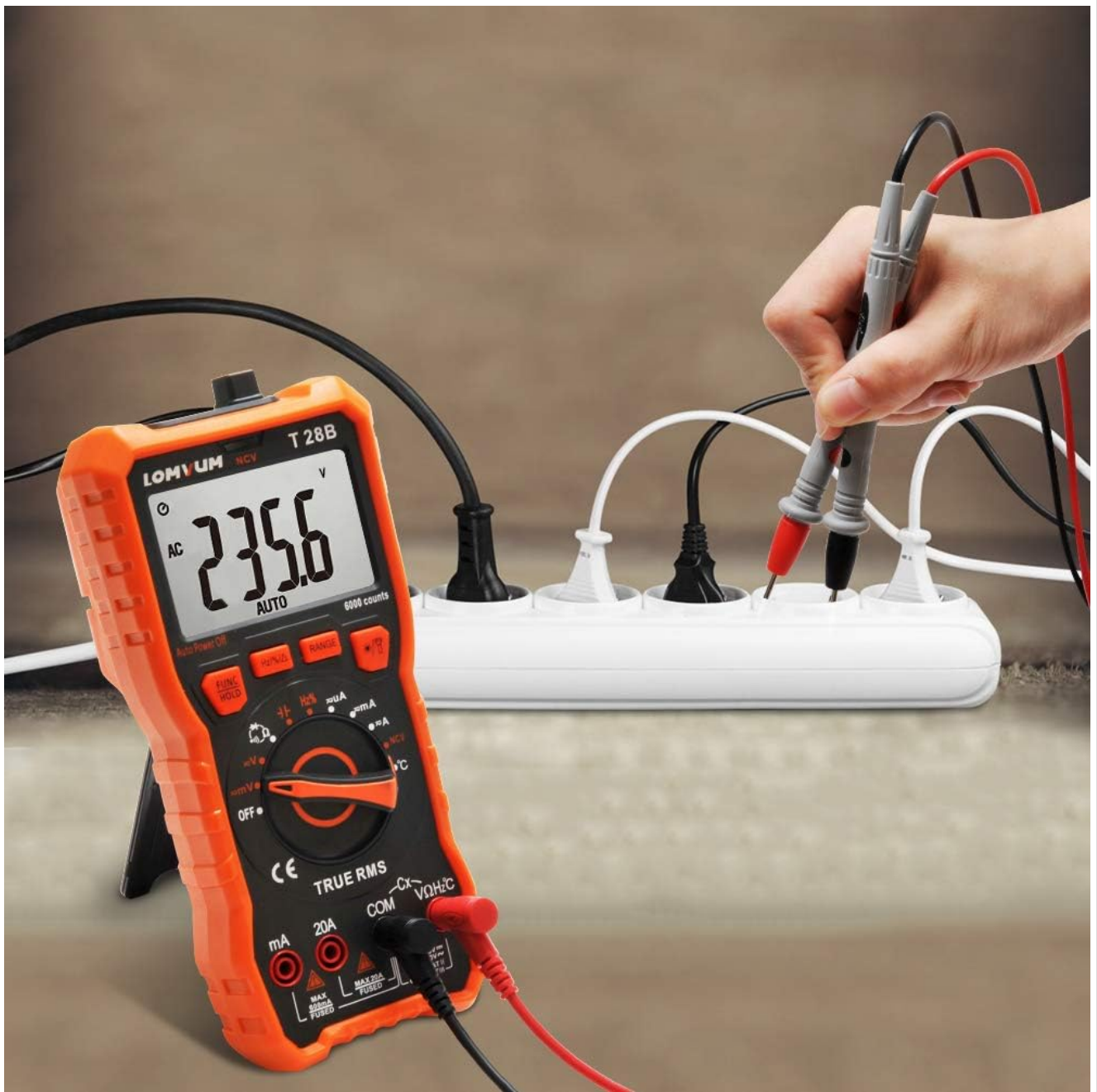
Image 7.2: The Lomvum T28B Multimeter performing a Non-Contact Voltage (NCV) test near a power strip to detect live wires.
