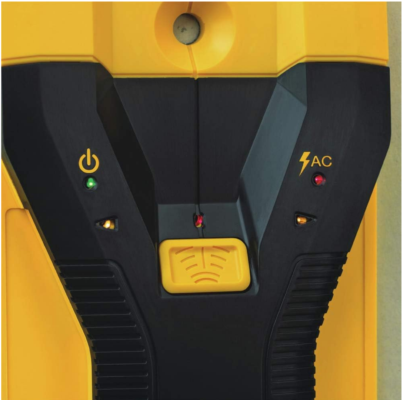
Image: Close-up of the stud finder's indicator lights, showing the AC detection warning.
